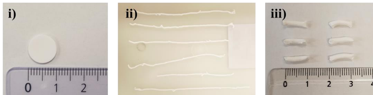
Figure V-2. Photographs of the pelletized (i) and extruded UiO-66-SO 3 H-W before (ii) and after cutting and drying (iii).
