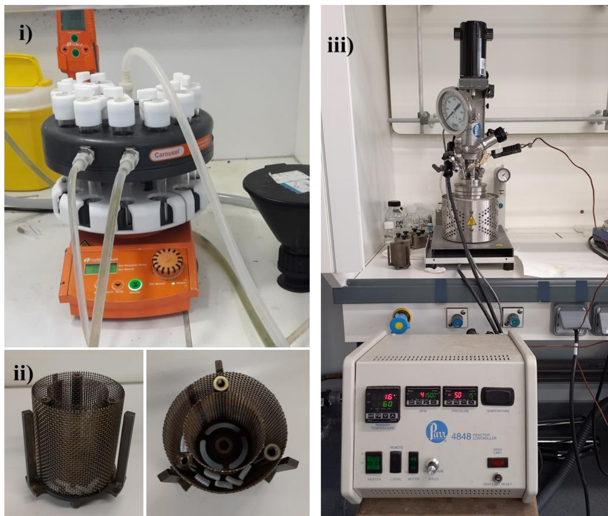
Figure II-8. Setups used to perform catalytic tests: Carousel Station (i) as well as the catalyst basket with the catalyst inside (ii), and the batch reactor Paar (iii).
