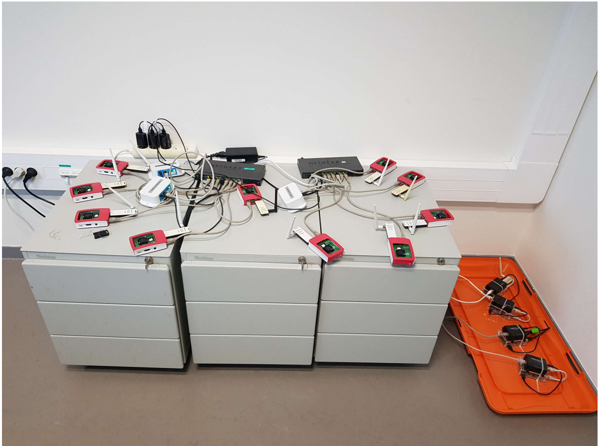
Fig. 4.10: Cluster of 10 Raspberry Pi with WiFi drivers, connected to a Walt server.
