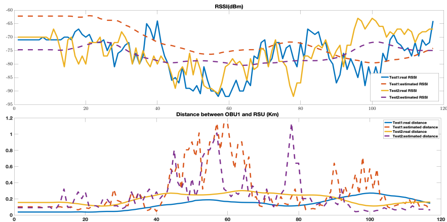
Fig. 7.6 Test 1 and 2 with RSU's RSSI estimation on V2I communication
