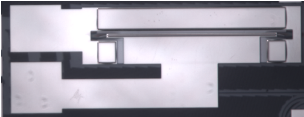
Figure 4.41: Microscope image of the fabricated III-V/Si DBR laser.
