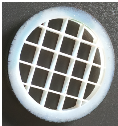
Figure 9 – Plastic grid positioned inside the tube to prevent the facings from bending. It adds a 0.89 mm shift due to its shoulder.
