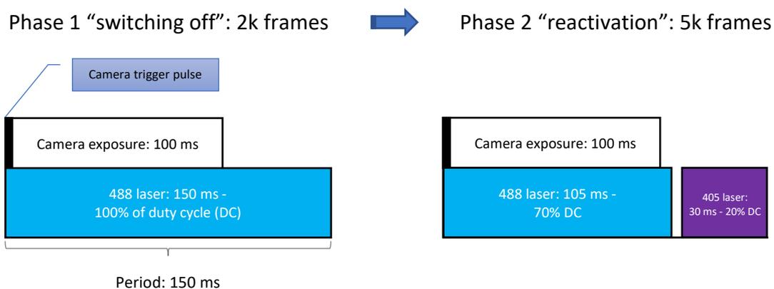
Figure S20: Illumination scheme employed in single-molecule experiments at CT. During 2000 frames a 488 nm laser was used to switch off the rsEGFP2 molecules and enter the single-molecule regime. During the second phase (5000 frames), a 405 nm laser was added to reactivate the molecules (after the camera exposure to not interfere with image readout).
