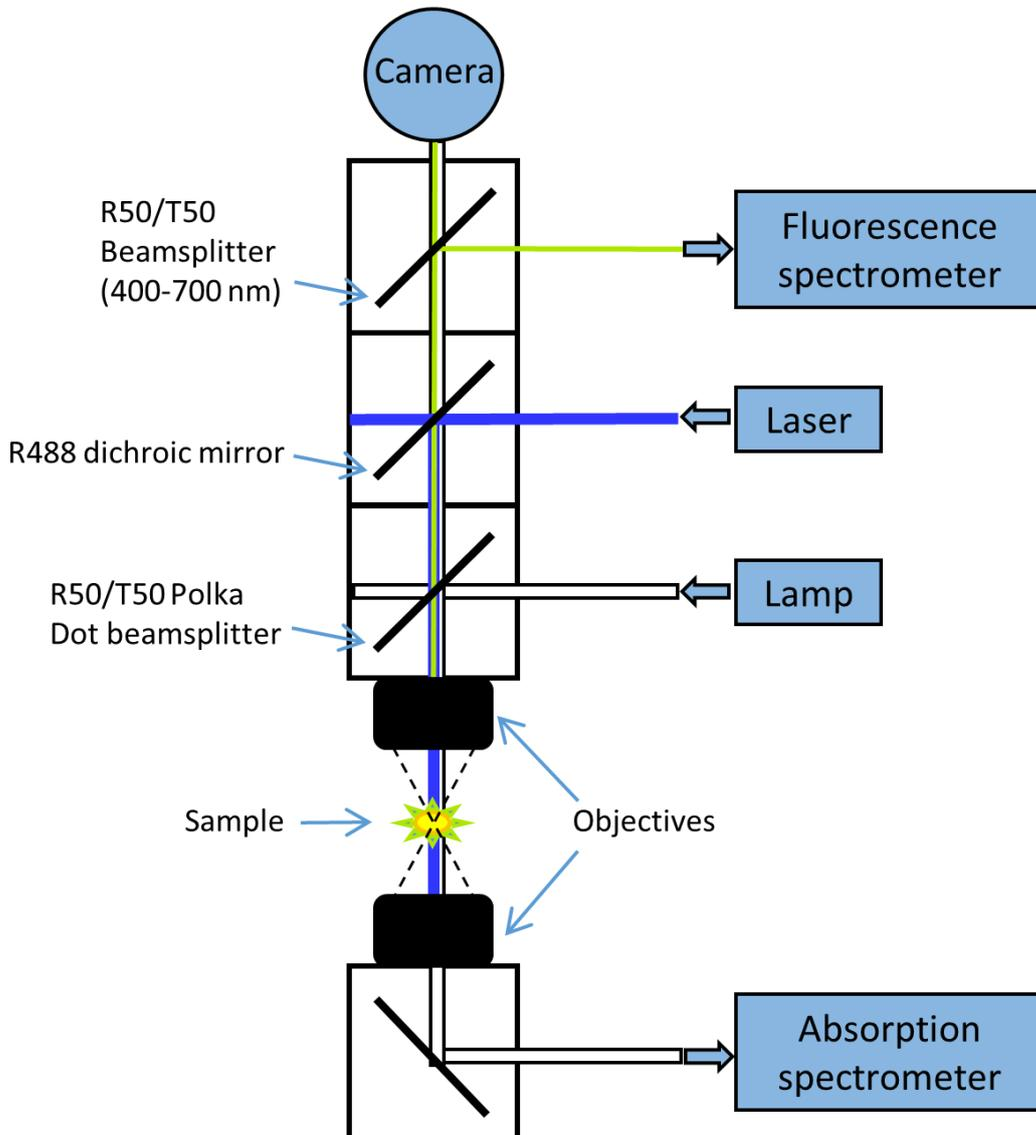
Figure 27: Microspectrophotometer setup used for this work.
