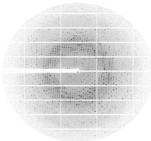
*Figure 22: Diffraction pattern collected at the ESRF. The thick white line in the middle is caused by the shadow of the beam blocker, which protects the detector from too intensive light of the central spot.*
