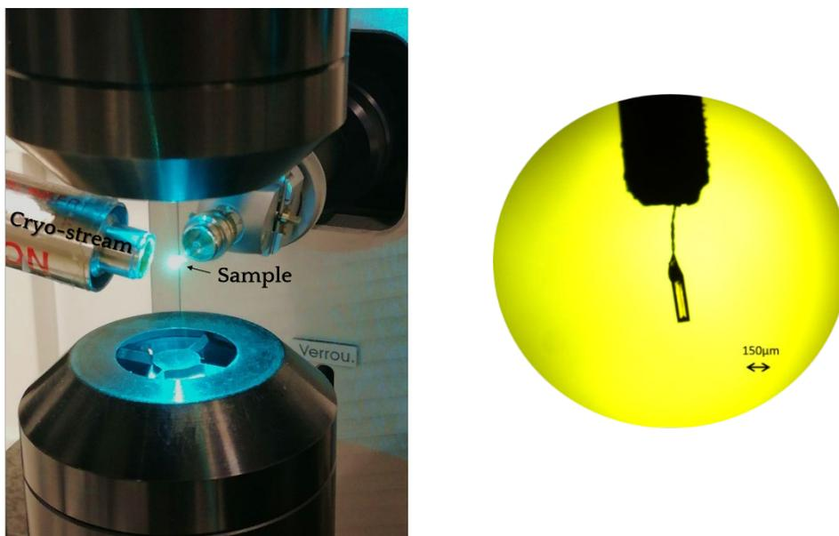
*Figure 26: An rsEGFP2 crystal in a silicon loop (zoomed in on the right) is placed between two objectives at the microspectrophotometer and is cooled by a cryo-stream. It fluoresces green upon illumination with 488 nm laser light.*
