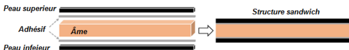
Figure V.1 : Constitution des structures sandwichs [7].
