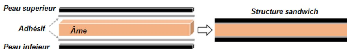
Figure V.1 : Constitution des structures sandwichs [7].
