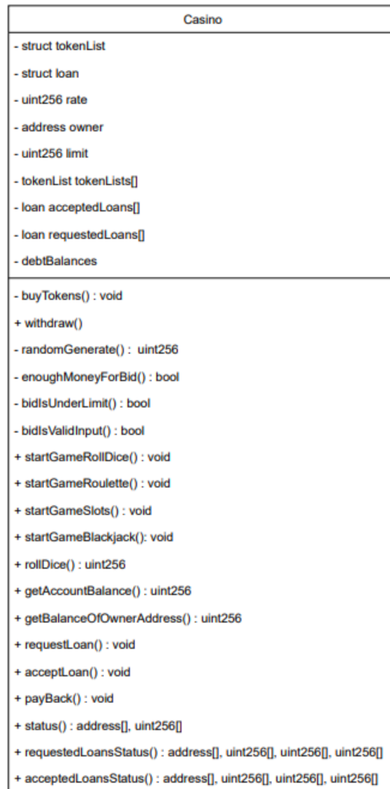
FIGURE B.2: Class Diagram: Gaming Platform
