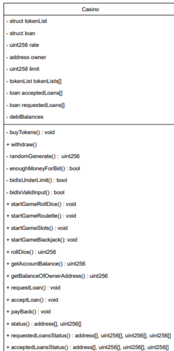
FIGURE B.2: Class Diagram: Gaming Platform
