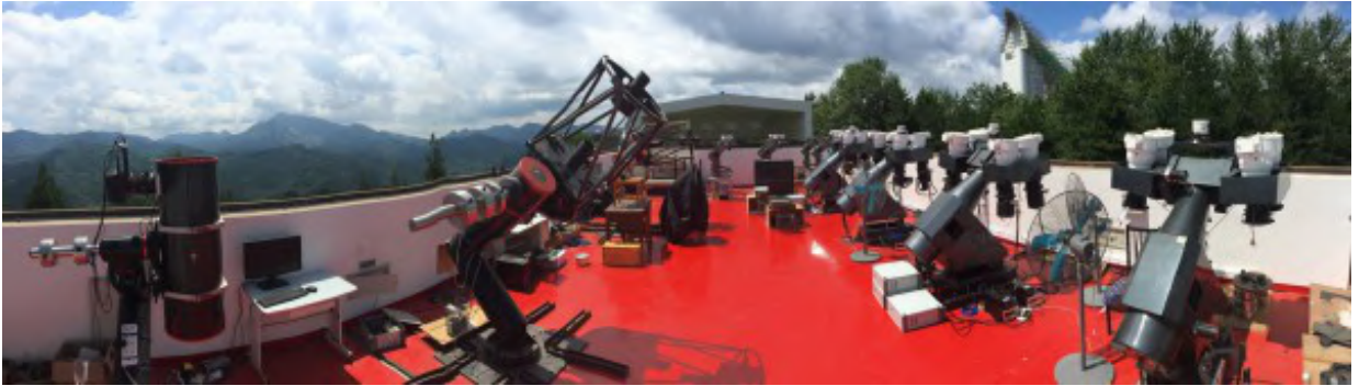
FIGURE 2.5. Panoramic view of GWAC installation at Xinglong Observatory (Beijing, China) showing 4 GWAC-A mountings (right) and the 60 cm and 30 cm telescopes (left). Credit: NAOC
