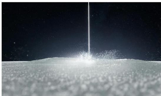
Figure 2: Laser powder bed fusion of plastic powder in an SLS [5].
