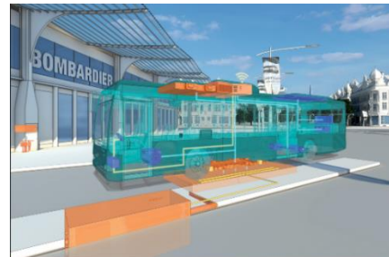
Figure 1.14 Bombardier RIPT charger for buses [29]
