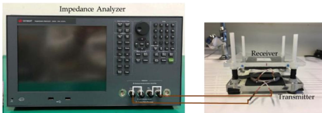
(a) Measurement of the self-inductance of the transmitter
