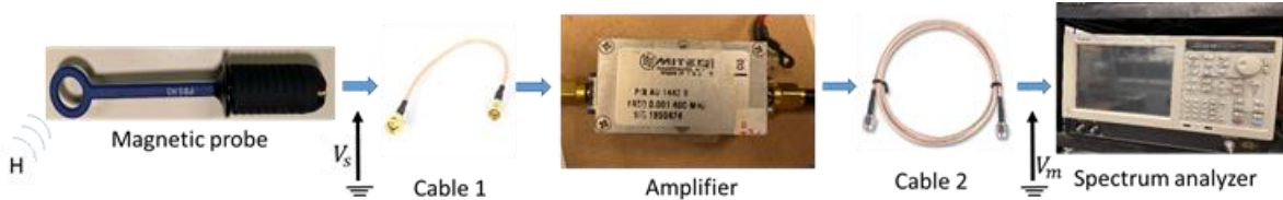
Figure 2.8 Measurement chain for the performance factor
