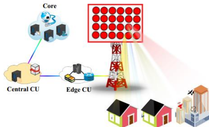
Figure 1-13. FWA network using Multiple Input Multiple Output and beamforming [3]
