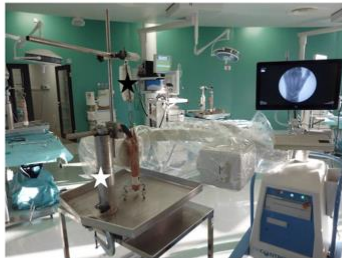
Fig. 1. Installation. The wrist is upright on a traction power (white star). The traction force is controlled by a dynamometer (black star). A fluoroscope is installed horizontally.
