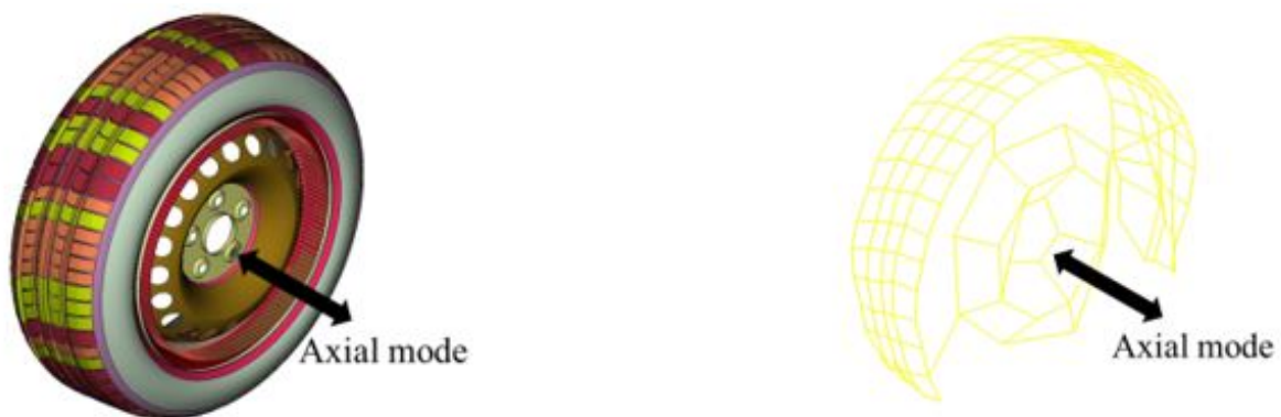
Figure A.1: Mode shape for Eigen mode 1 (66 Hz) – (left) from simulation and (right) from test.
