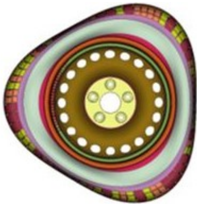
Figure A.4: Mode shape for Eigen mode 4 (146 Hz) – (left) from simulation and (right) from test.
