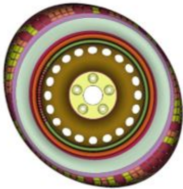
Figure A.3: Mode shape for Eigen mode 3 (118 Hz) – (left) from simulation and (right) from test.
