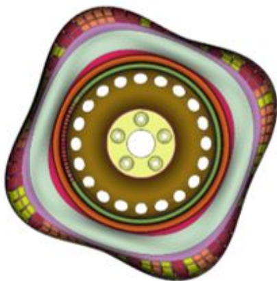
Figure A.5: Mode shape for Eigen mode 5 (171 Hz) – (left) from simulation and (right) from test.
