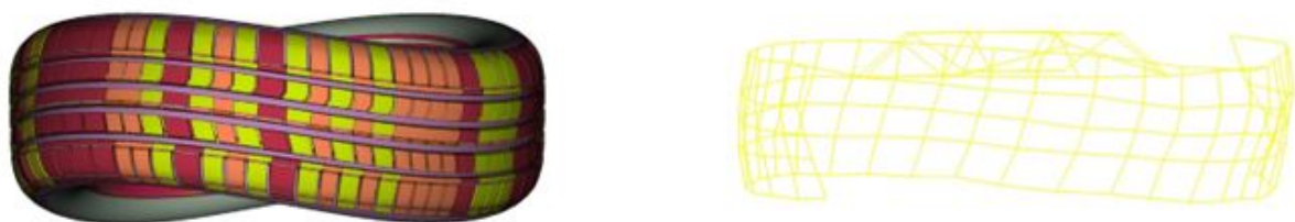
Figure A.2: Mode shape for Eigen mode 2 (100 Hz) – (left) from simulation and (right) from test.
