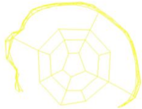
Figure A.3: Mode shape for Eigen mode 3 (118 Hz) – (left) from simulation and (right) from test.
