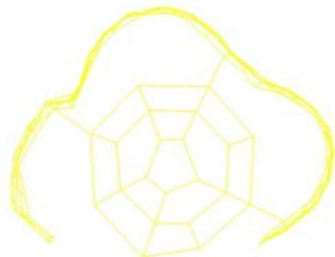
Figure A.5: Mode shape for Eigen mode 5 (171 Hz) – (left) from simulation and (right) from test.
