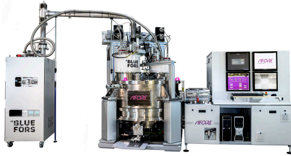
Figure 4.1: Cryogenic probe station designed for measurements of 300 mm wafers.
