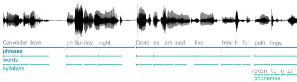
Figure 1.2: Example of speech input divided into its linguistic constituents at different time scales. On top, the speech waveform of the sentence “Can you believe on Sunday night, David examined five beautiful paintings”. Following respectively, the phrasal segmentation, the words segmentation, the syllabic segmentation, and a phonemic segmentation for the last word of the sentence “paintings”. Image is taken from (Keitel et al., 2018).
