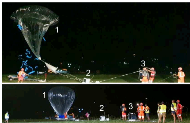
(b) Two consecutive photos taken at the release of the balloon: the lower one shows the balloon still on the table (1) and the flight chain still on the ground. The latter is made up of the CNES EUROS gondola (2) in charge of flight safety, then the ZEPHYR gondola (3) which carries the various scientific instruments listed in the table (1.1). The top photo shows the moment when the balloon is released. It will soon carry the whole flight chain to the stratosphere.
