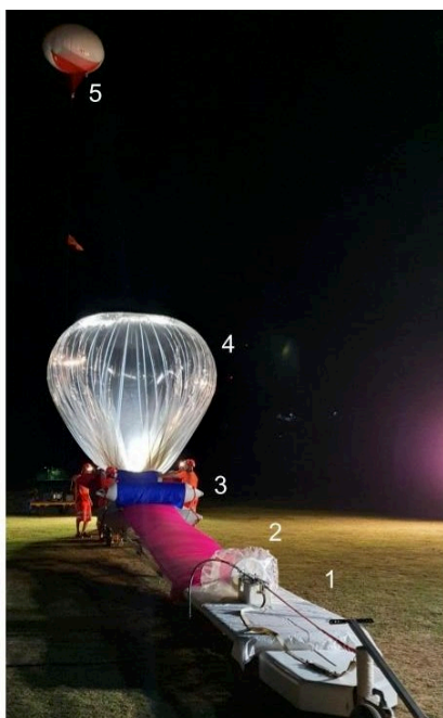
(a) The last step before the launch of the balloon is its inflation. The balloon has previously been laid on the table (1). It is inflated (4) with a fixed amount of gas through its valve (2), that does not fill it completely (see explanation in text). The rest of the balloon is still folded on the table, under the pink layer and a weight (3) separates the inflated part from the rest and prevents the balloon from flying away. Note the red balloon at the top left (5), used to know the local wind at the airport and to approve the launch (the wind must be quite weak near the surface).
