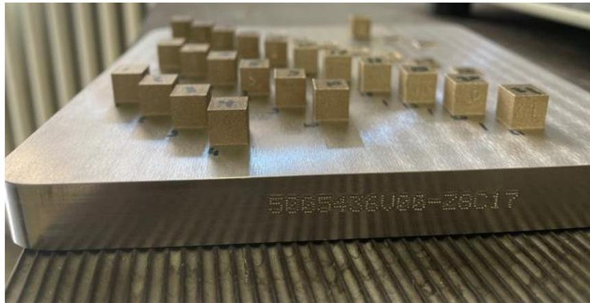
*Figure 6.9 Top and side views of a standard build plate with built cubes ( $10 \times 10 \times 10 \text{ mm}^3$ ) printed atop it*
