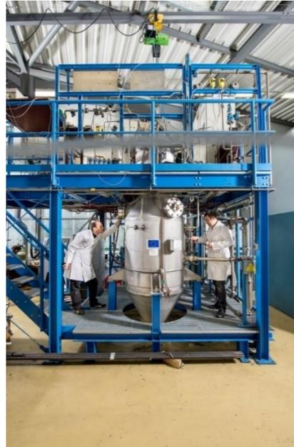
Figure 3.1 a) Schematic of a gas atomization chamber b) gas atomizer in UTBM lab
