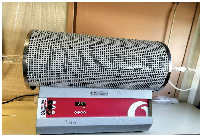
Figure 2.2.2 : The Carbolite tubular furnace used for calcination.
