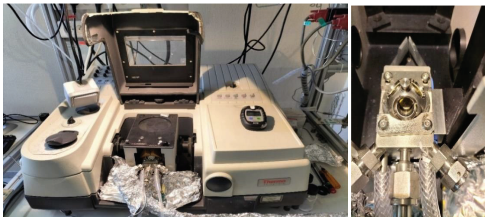
Figure 2.3.5 : The Nicolet 8700 instrument (left) and the Harrick cell TM (right).
