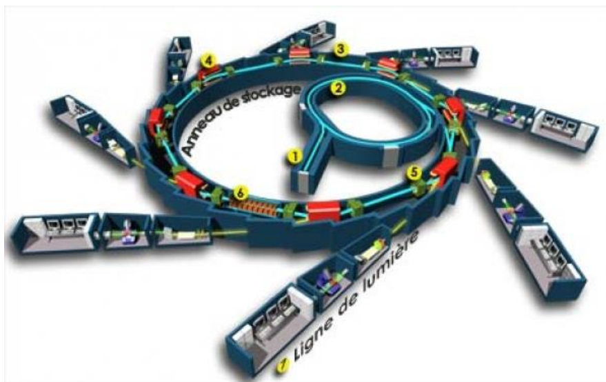
Figure 3.1 A schematic diagram of a third-generation synchrotron radiation centre. (Image taken from website of SOLEIL)
