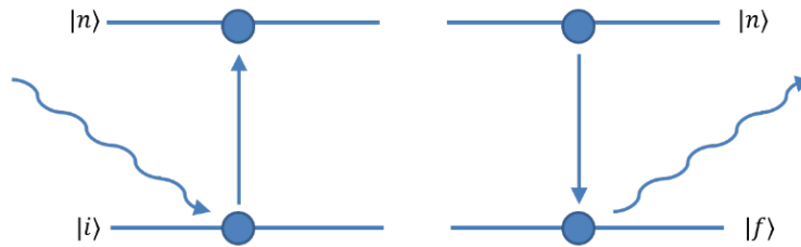
Figure 2.7 Diagram of resonant x-ray absorption showing each energy level with the electronic quantum states.
