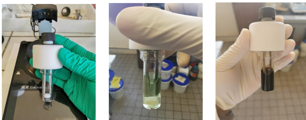
Figure 9. Left. Electrode, Mg and Ni form. Middle. The mixture before reaction. Right. The mixture after reaction.
