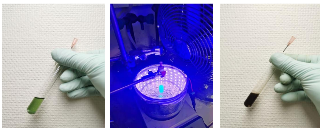
Figure 16 Mixture before reaction (Left); Photoreactor bed (Middle); Mixture after reaction (Right).
