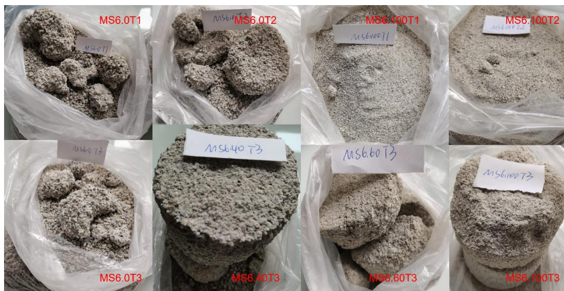
Fig. 6.12 Treated specimens of various sands with various cementation levels after cyclic triaxial tests
