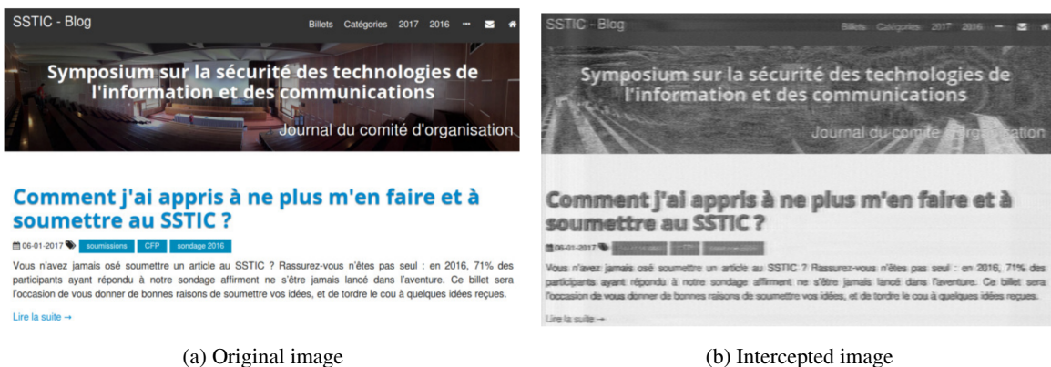
Figure 1.5 – TEMPEST exploitation example: interception of a DVI video stream [RD18]
