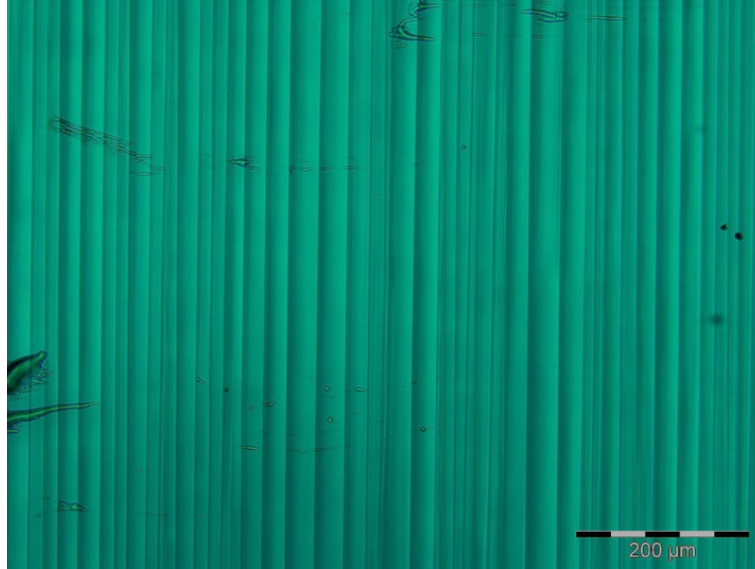
Figure I.11: Optical microscope image of a CTO single crystal. Parallel domains are visible by birefringence.
