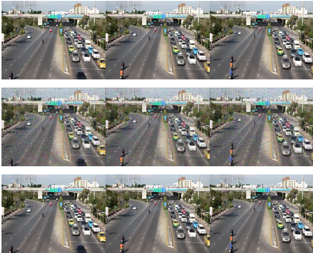
Figure 8.18: Frames of the original video (top), frames of the blurred and noisy video (center), frames of the restored video(bottom).
