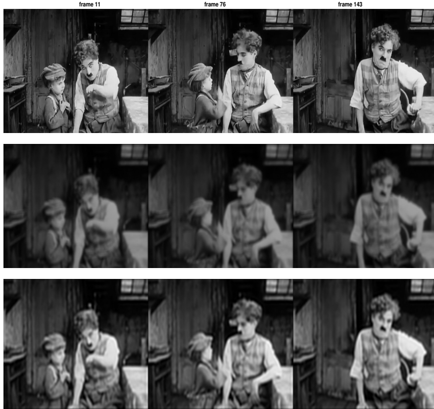
Figure 8.11: Original frames (top), blurred and noisy frames with SNR = 4.85 (center) and restored frames with SNR = 15.73 in 92 s (bottom).
