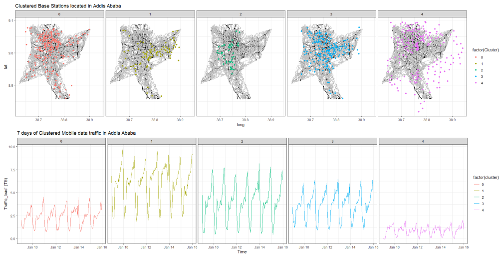
Figure 5.20: UMTS radio nodes clustered based on their traffic patterns using the DEC_MT arrangement. The clustering was performed using DEC and the time domain centroids are estimated by training a multi-tasking neural network from scratch
