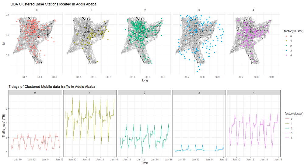
Figure 5.17: UMTS radio nodes clustered based on their traffic patterns using DBA K-means
