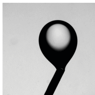
Figure 3.7: Droplet of Ethyl palmitate in water highlighting the measuring procedure of the interfacial tension in the pendant drop method.
