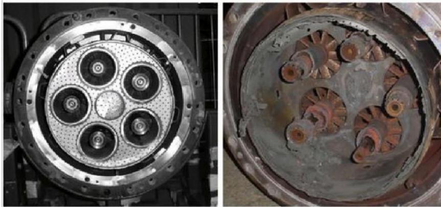
**Figure 1.5:** Destructive impact of CIs; Burner nozzle before (left) and after (right) a CI event
