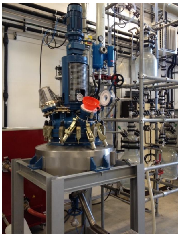
Fig. 2.6 Set-up for the alkaline extraction on SCB in 100 L stainless steel-lined vessel.
