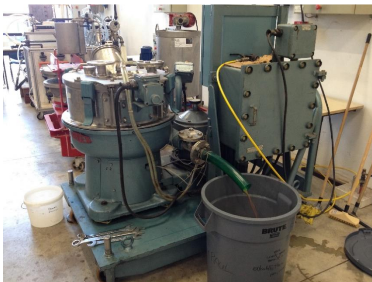
Fig. 2.7 Solid residue/alkaline extract separation using a top-discharge vertical basket centrifuge (RC 50 PX R, Rousselet) equipped with a 5 \mu\text{m} polypropylene bag.
