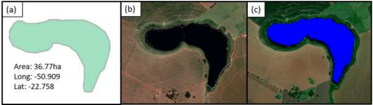
Figure III-5: Example of the stratified analysis for an unnamed water body. (a) Shape file with its area and coordinates; (b) high resolution imagery; and (c) overlaid water mask for June 2020.
