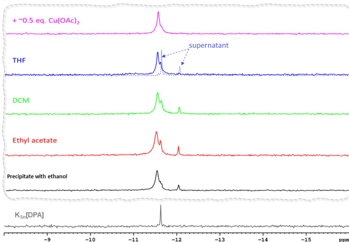
Figure 3-13 The  $^{31}\text{P}$  NMR of  $\text{K}_{\text{Sn}}[\text{DPA}]@\text{Cu}(\text{OAc})_2$  after the treatment with ethanol (black), ethyl acetate (red), dichloromethane (green) and THF (blue); add  $\sim 0.5$  eq.  $\text{Cu}(\text{OAc})_2$  based on the THF treatment (purple).
