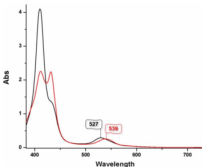
Figure 4-17 The UV-vis spectrum of 0.08mM Co-TPP to detect the production of NO in the photoreduction of  $TBANO_2$  (40 mM) with  $D_{V3DPA}Cu(OAc)$  (0.5 mM) in the presence of  $PhCOOH$  (40 mM).
