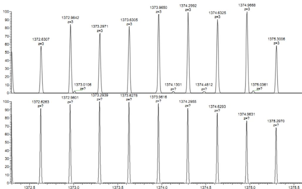
Figure 4-39 The ESI-MS of  $D_{V3DA}$  which gives the formular  $\{H_3[P_2V_3W_{15}O_{62}(Tris-DA)]\}^{3-}$
