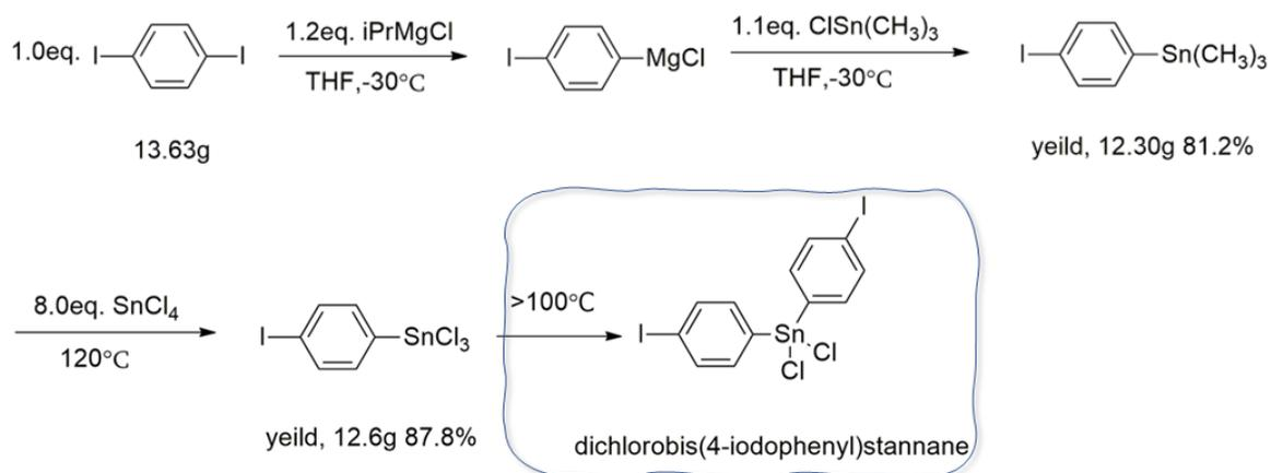
*Scheme 3-1 The synthesis route of I-iodo-4-(trichlorotin) Benzene and the proposal dimerization.*
