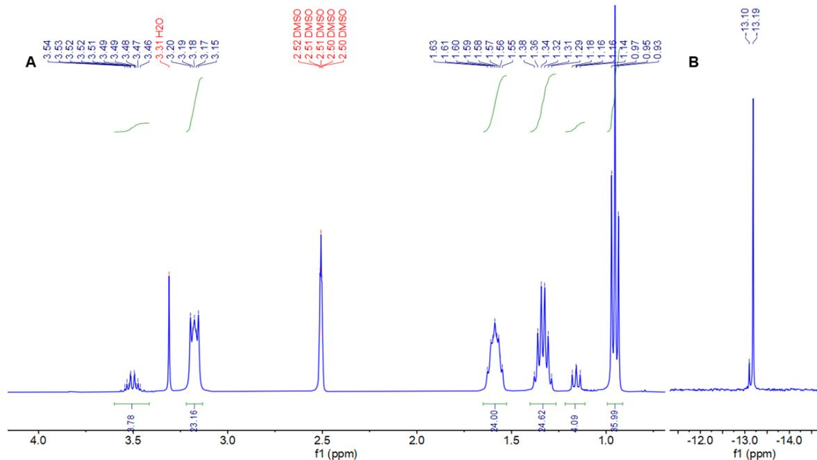
Figure 3-41 The  $^1\text{H}$  NMR (A) and  $^{31}\text{P}$  NMR (B) of  $\text{KSi}[\text{N}_3]\text{-2}$  in DMSO.
