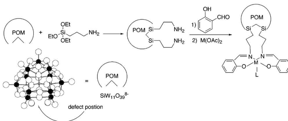
Figure 1-21 Synthetic Pathway for the preparation of the M-Salen-POM Compounds,  $M = \text{Mn}, \text{Co}, \text{Ni}$  and  $\text{Pd}$ .<sup>42</sup>
