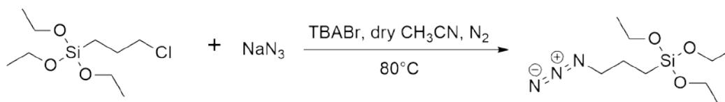
Scheme 3-6 The synthesis of 3-azidopropyl triethoxysilane.
