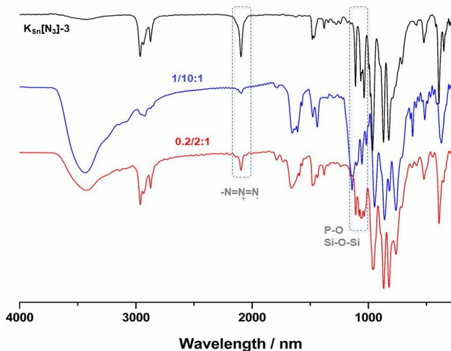
Figure 3-25 The IR of the resulting product with the ratio of  $\text{CuSO}_4$  /sodium ascorbate to  $\text{K}_{\text{Si}}[\text{N}_3]\text{-3}$  = 1/10:1(blue)and 0.2/2:1(red) in mixture solvent DMF/ $\text{H}_2\text{O}$ .
