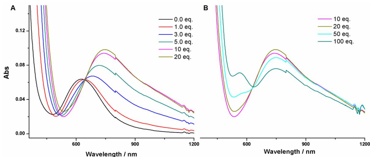
Figure 3-18 the UV-vis spectrum of 0.5 mM  $K_{Sn}[DPA]@Cu(OAc)_2$  in the present of A) 1, 3, 5, 10, 20 eq. and B) 10, 20, 50 and 100 eq.  $TBANO_2$ .
