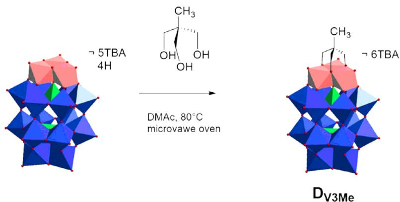
Scheme 4-6 The synthesis of  $TBA_6[P_2V_3W_{15}O_{62}(TrisMe)]$  ( $D_{V3Me}$ )
