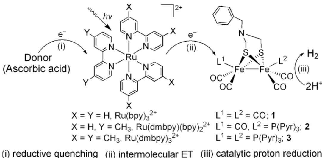
Figure 1-4 The Homogeneous Molecular Three-Component System for Photochemical H<sub>2</sub> Generation Catalyzed by [Fe-Fe]H<sub>2</sub>ase Active Site Mimics.<sup>16</sup>
