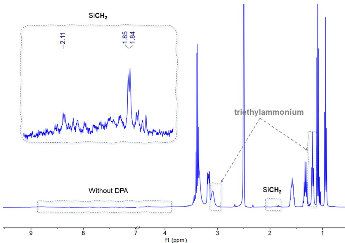
Figure 2-7 the  $^1\text{H}$  NMR of the resulting product with the addition of  $\text{Et}_3\text{N}$  as the base
