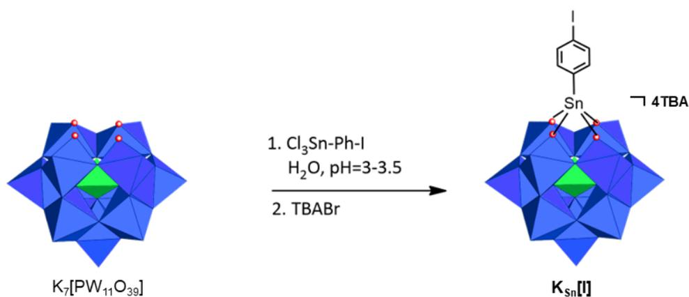
Scheme 3-3 The synthesis of  $\text{K}_{\text{Sn}}[\text{I}]$
