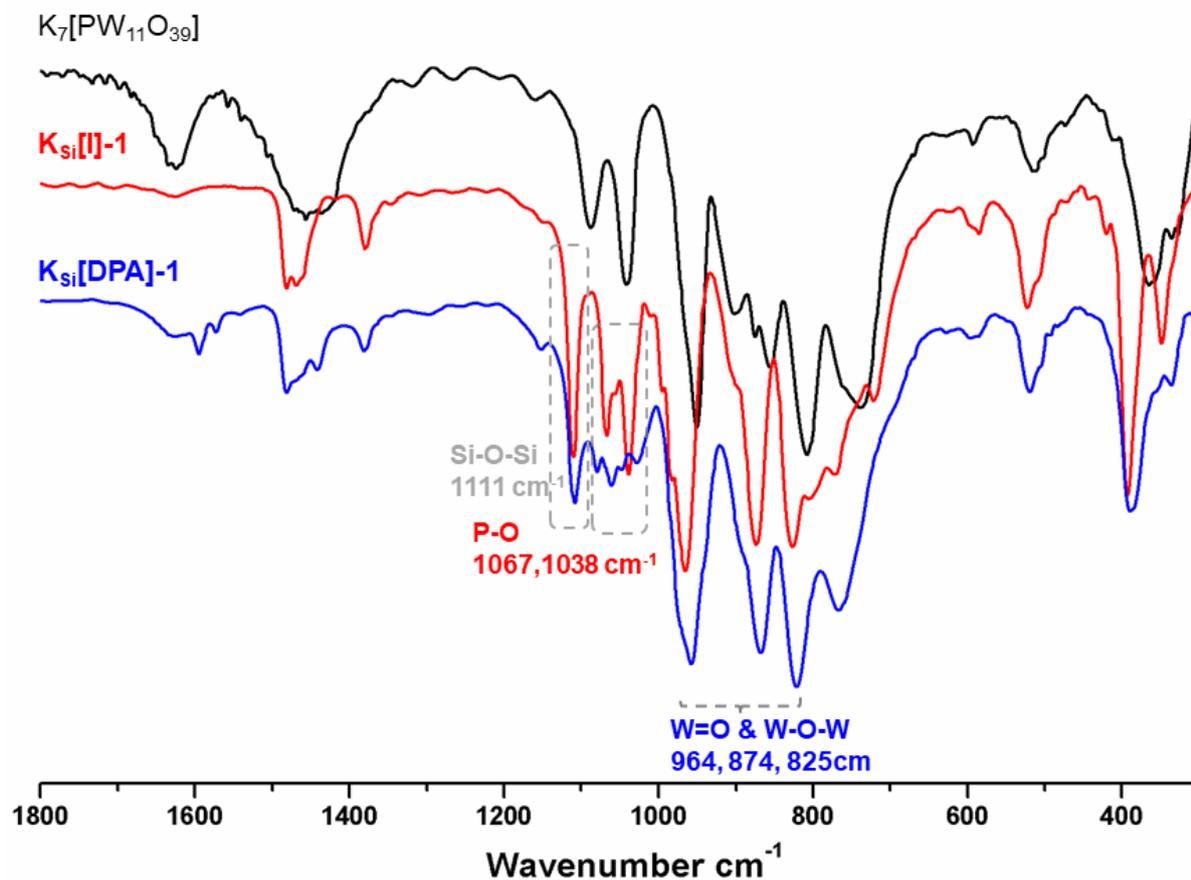
Figure 2-5 IR spectrum (KBr) of the  $K_7[PW_{11}O_{39}]$  (black),  $K_{Si}[I]-1$  (red), and the synthesized  $K_{Si}[DPA]-1$  (blue).
