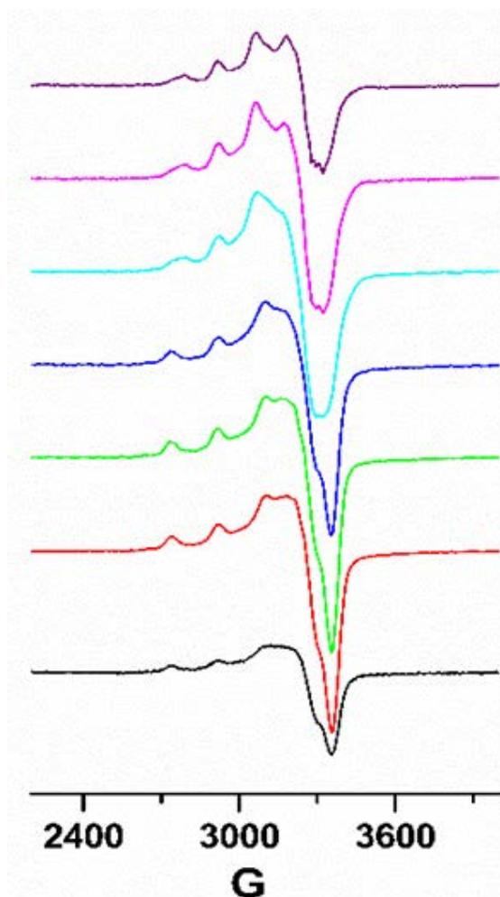
Figure 3-19 The EPR spectrum of 0.5 mM  $K_{Sn}[DPA]@Cu(OAc)_2$  in the presence of 0, 1, 3, 5, 10, 20 and 50 of  $TBANO_2$
