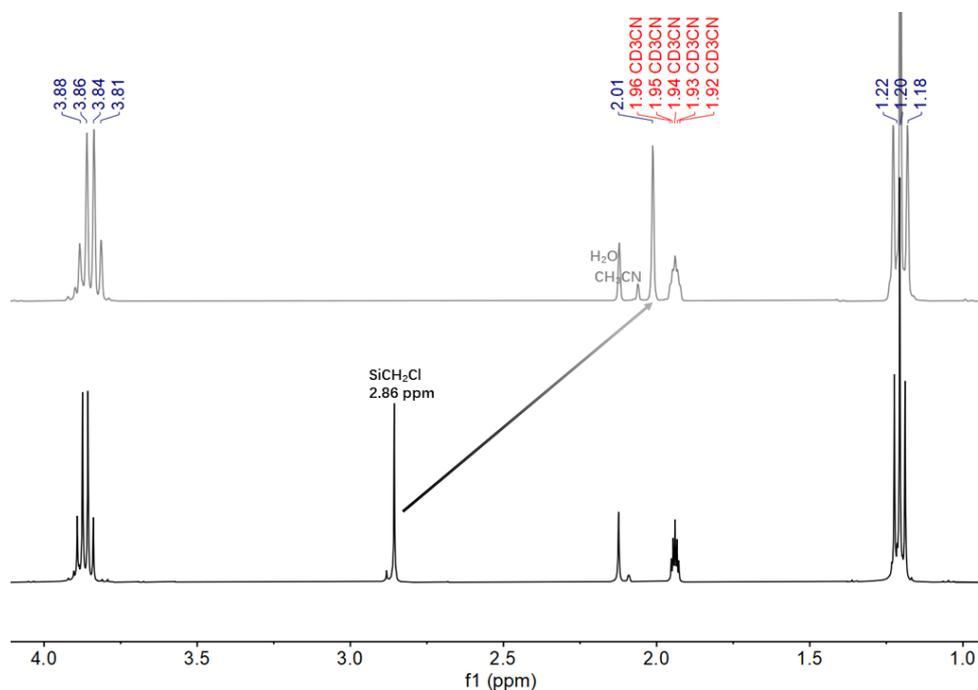
*Figure 2-1 <sup>1</sup>H NMR spectrum of triethoxy(iodomethyl)silane (gray) and triethoxy(chloromethyl)silane (black) in CD<sub>3</sub>CN.*
