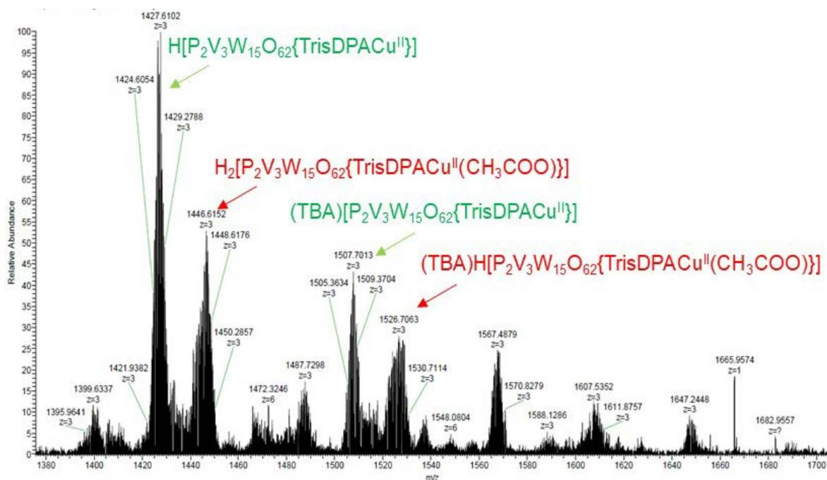
Figure 4-10: ESI-MS spectrum and attribution of various peaks of trianionic species derived from the  $D_{V3DPA}Cu(OAc)$  anion
