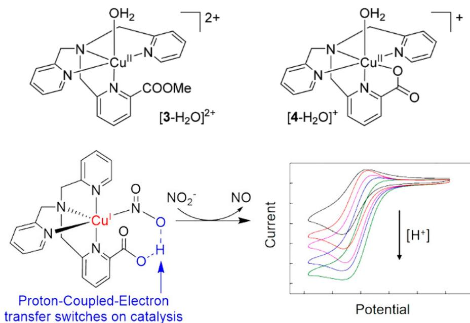
Figure 1-5 The two bioinspired tripodal N-donor Cu-complexes and the proposal Proton-Coupled-Electron transfer mechanism for the electrocatalytic reduction process of nitrite.<sup>17</sup>
