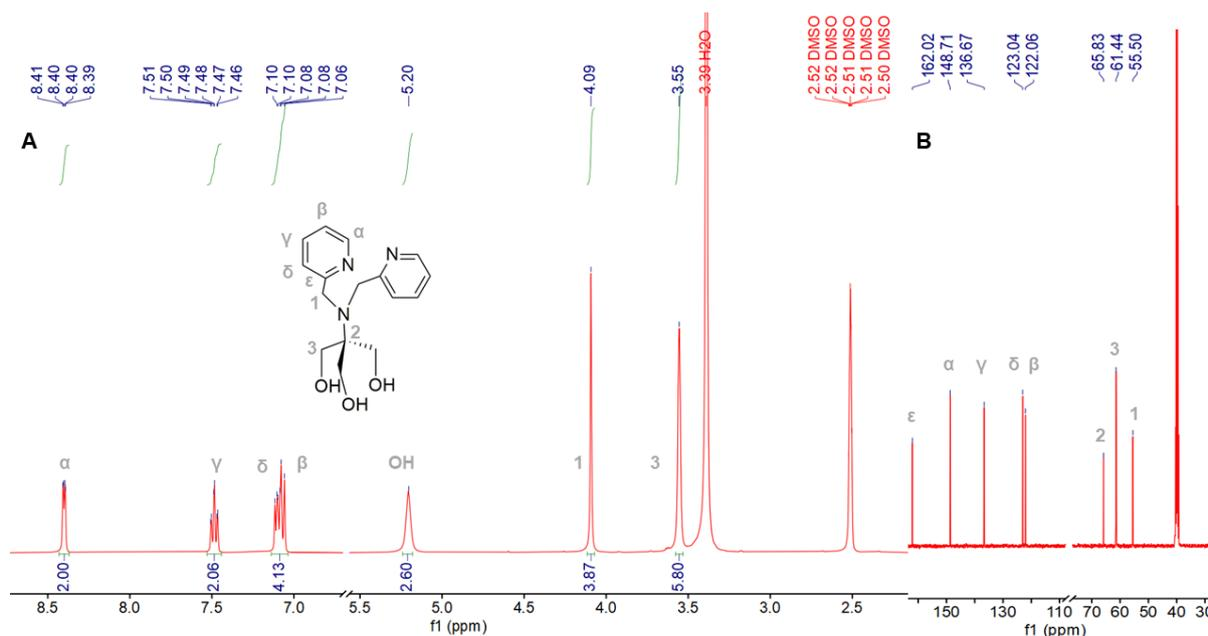
Figure 4-1 A)  $^1H$  NMR and B)  $^{13}C$  NMR of  $H_3Tris-DPA$  (in DMSO).
