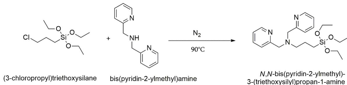
Scheme 2-9 The synthesis of *N,N*-bis(pyridin-2-ylmethyl)-3-(triethoxysilyl)propan-1-amine.
