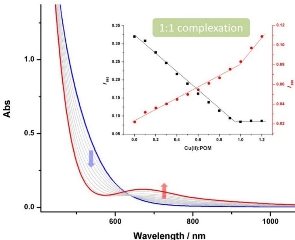
Figure 4-9: UV vis titration of  $D_{V3DPA}$  (1.0 mM) with increasing amount of  $Cu(OAc)_2$ .
