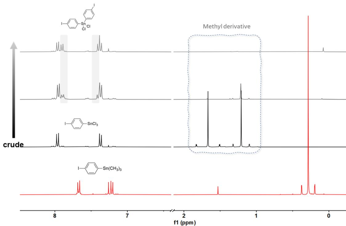
Figure 3-1  $^1\text{H}$  NMR monitor of the synthesis of 1-iodo-4-(trichlorotin) Benzene from 1-Iodo-4-(trimethyltin)benzene; and the distillation to remove the methyl derivatives.
