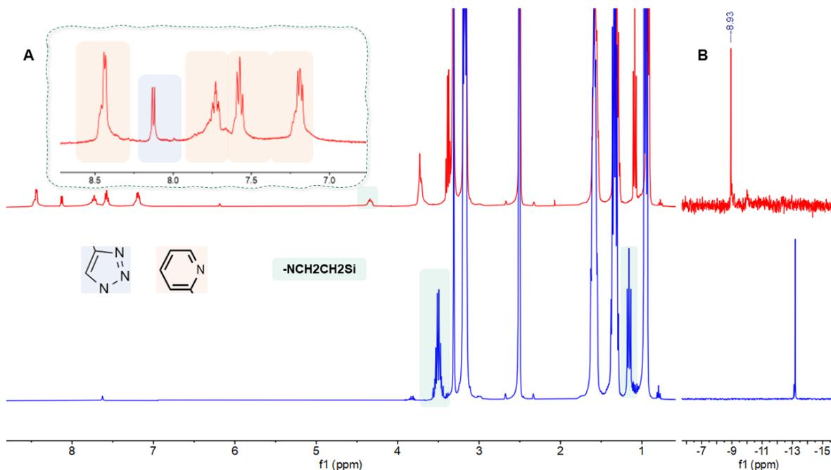
Figure 3-42 The  $^1H$  NMR (A) and  $^{31}P$  NMR (B) of  $(K_{Si}[N_3DPA]-2)$  (red) in DMSO.
