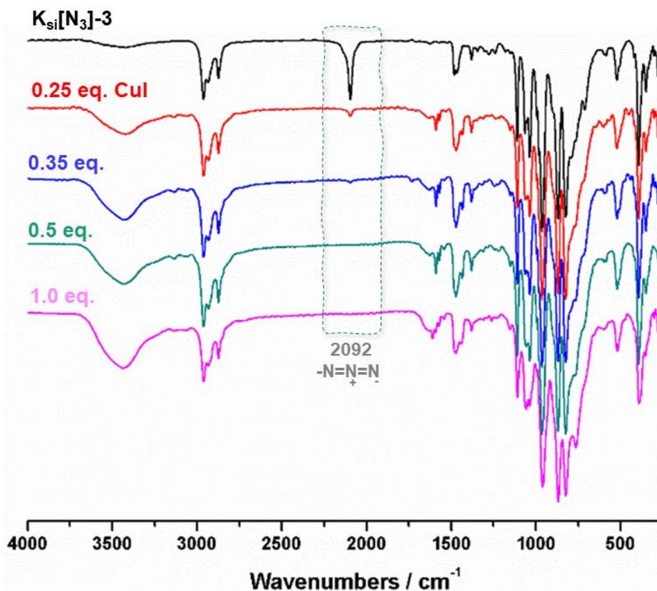
Figure 3-35 the optimization of the amount of CuI in the “click” reaction of  $K_{Si}[N_3]-3$  and propargyl-DPA.
