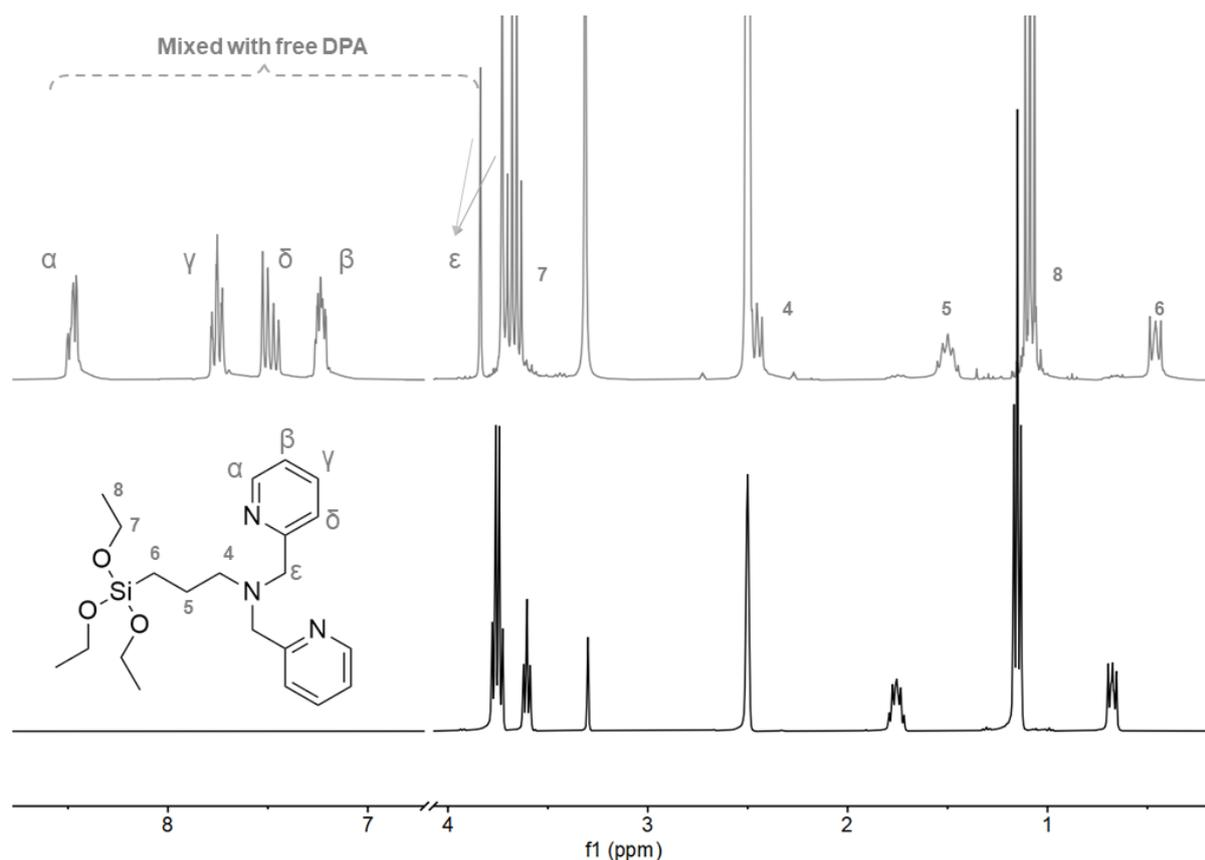
Figure 2-12 The evolution in  $^1\text{H}$  NMR of *N,N*-bis(pyridin-2-ylmethyl)-3-(triethoxysilyl)propan-1-amine (gray) from the reaction of (3-chloropropyl)triethoxysilane (black) and DPA.
