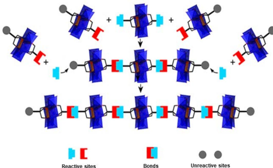
*Figure 1-16 Combinations possible with AA couplings (between two identical functional groups) and AB couplings (between two different functional groups) shown for Anderson POMs.<sup>53</sup>*
