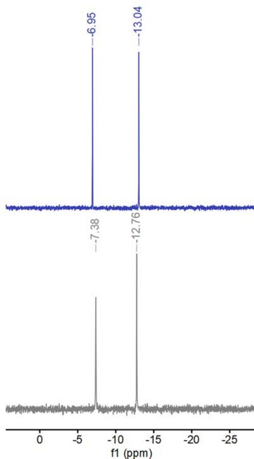
Figure 4-2 Comparison of the  $^{31}P$  NMR ( $CD_3CN$ ) in the synthesis of  $D_{V3DPA}$  (blue) from  $D_{V3}$  (gray).
