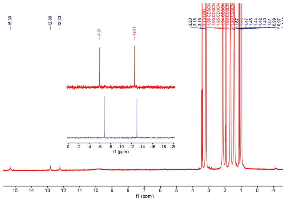
Figure 4-12 The  $^1\text{H}$  NMR ( $\text{CD}_3\text{CN}$ ) of the  $\text{D}_{\text{V}_3\text{DPA}}\text{Cu}(\text{OAc})$ ; insert: The variation of the  $^{31}\text{P}$  NMR ( $\text{CD}_3\text{CN}$ ) in the synthesis of  $\text{D}_{\text{V}_3\text{DPA}}\text{Cu}(\text{OAc})$  (red) from  $\text{D}_{\text{V}_3\text{DPA}}$  (navy blue).
