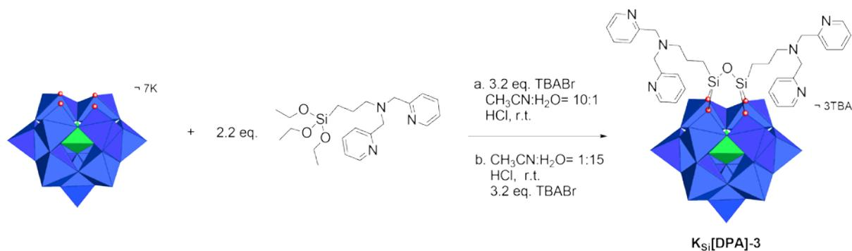
Scheme 2-11 The direct-functionalization of  $\text{K}_{\text{Si}}[\text{DPA}]-3$ .
