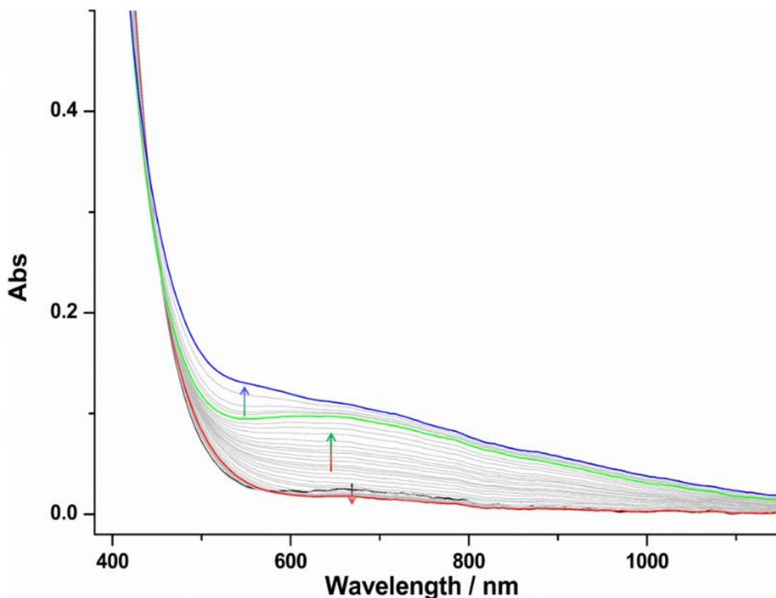
Figure 4-16 : UV-vis evolution upon electrochemical reduction of a  $0.2 \text{ mmol}^{-1}$  solution of  $D_{V3DPA}Cu(OAc)$  in  $CH_3CN / 0.1M TBABF_4$  electrolyte from  $0.2 \text{ V/SCE}$  to  $-1.5 \text{ V/SCE}$ . The arrows describe the successive evolutions upon change in the signature of the reduced species, with stationary forms highlighted in red ( $1e^-$  reduced signature), green ( $2e^-$ ), blue ( $3e^-$ ).
