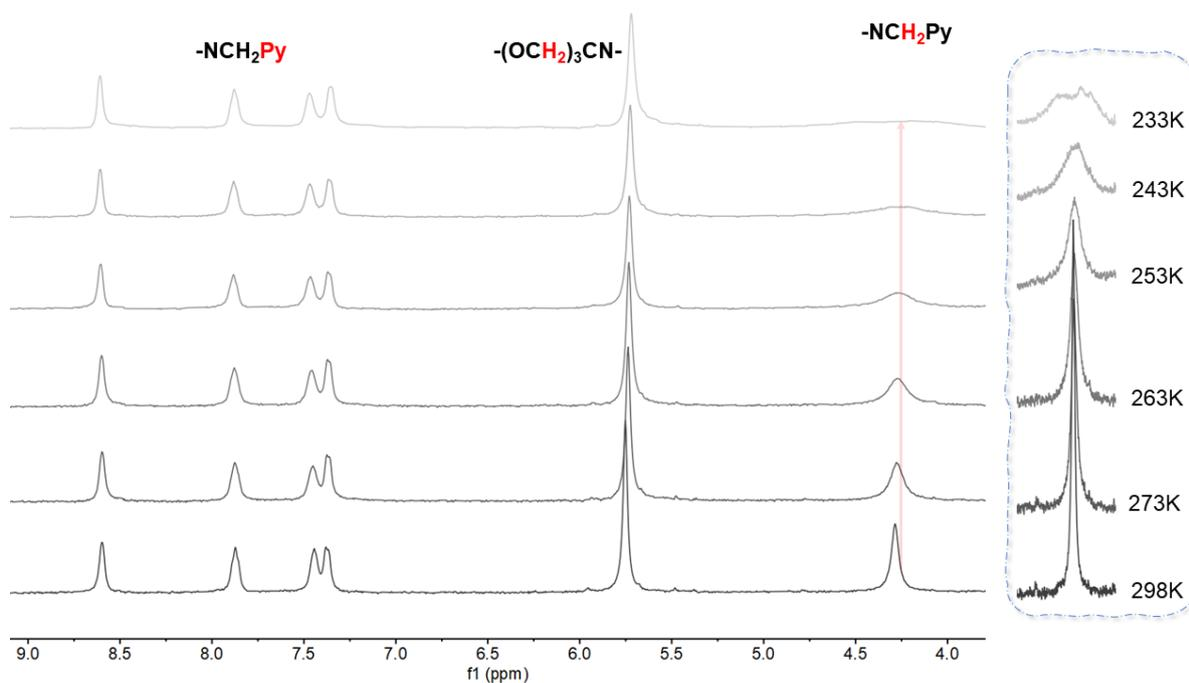
Figure 4-14 Evolution of the  $^1H$  NMR of  $D_{V3DPA}Cu^I$  in  $CD_3CN$  with temperature.
