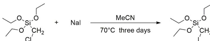
*Scheme 2-5 The synthesis of the triethoxy(iodomethyl)silane*
