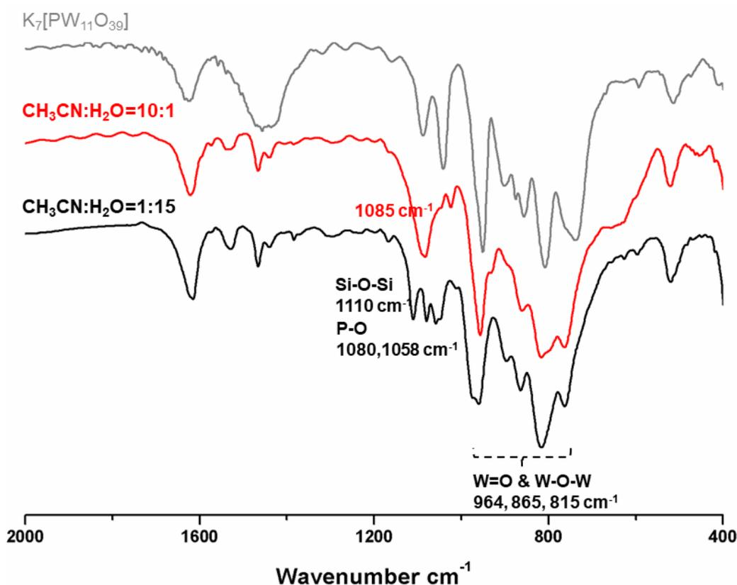
Figure 2-14 IR of the direct-functionalization of  $\text{K}_{\text{Si}}[\text{DPA}]-3$  in solvent  $\text{CH}_3\text{CN}:\text{H}_2\text{O}=10:1$  (red) and  $\text{CH}_3\text{CN}:\text{H}_2\text{O}=1:15$  (black) compared to the  $\text{K}_7[\text{PW}_{11}\text{O}_{39}]$  (gray).
