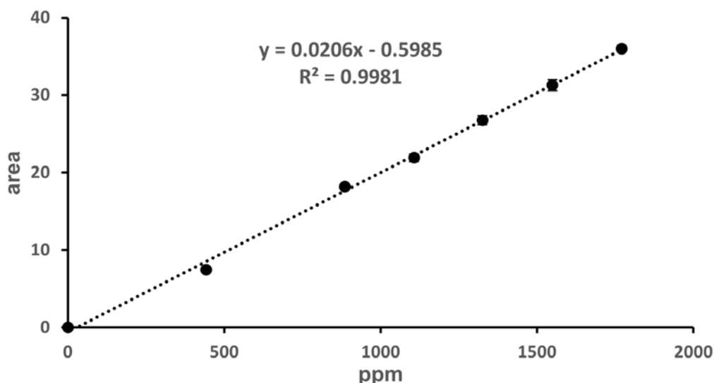
Figure 4-36 The GC calibration curve of NO produced from the reduction of sodium nitrite with ascorbic acid in the presence of glacial acetate acid.
