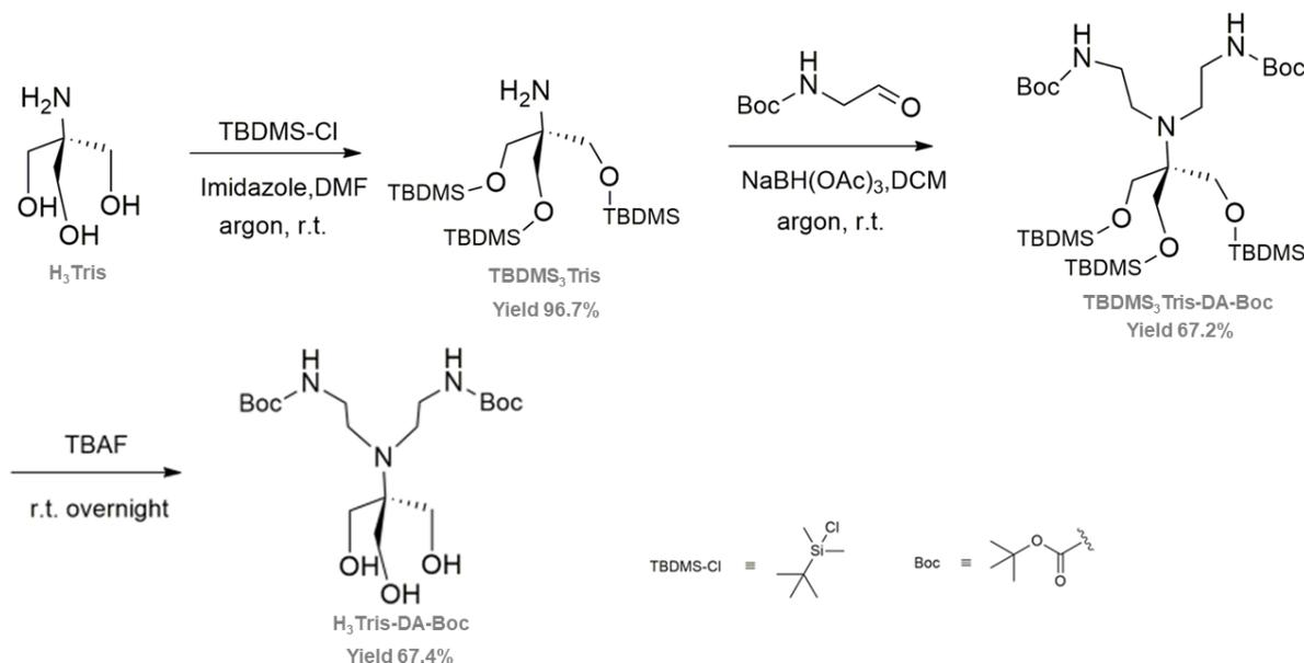
*Scheme 4-3 The synthesis route of the di-tert-butyl (((1,3-dihydroxy-2-(hydroxymethyl)propan-2-yl)azanediyl)bis(ethane-2,1-diyl))dicarbamate ( $H_3$ Tris-DA-Boc).*
