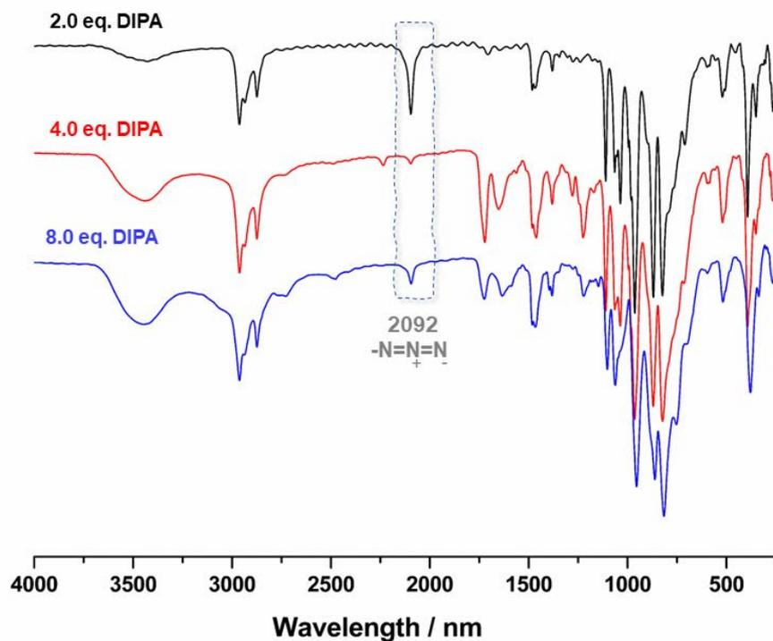
Figure 3-28 IR monitor of the “click” between  $K_{Si}[N_3]-3$  and methyl propiolate in the presence of different amount of DIPA 2.0 eq. (black), 4.0 eq. (red) and 8.0 eq (blue) at room temperature.
