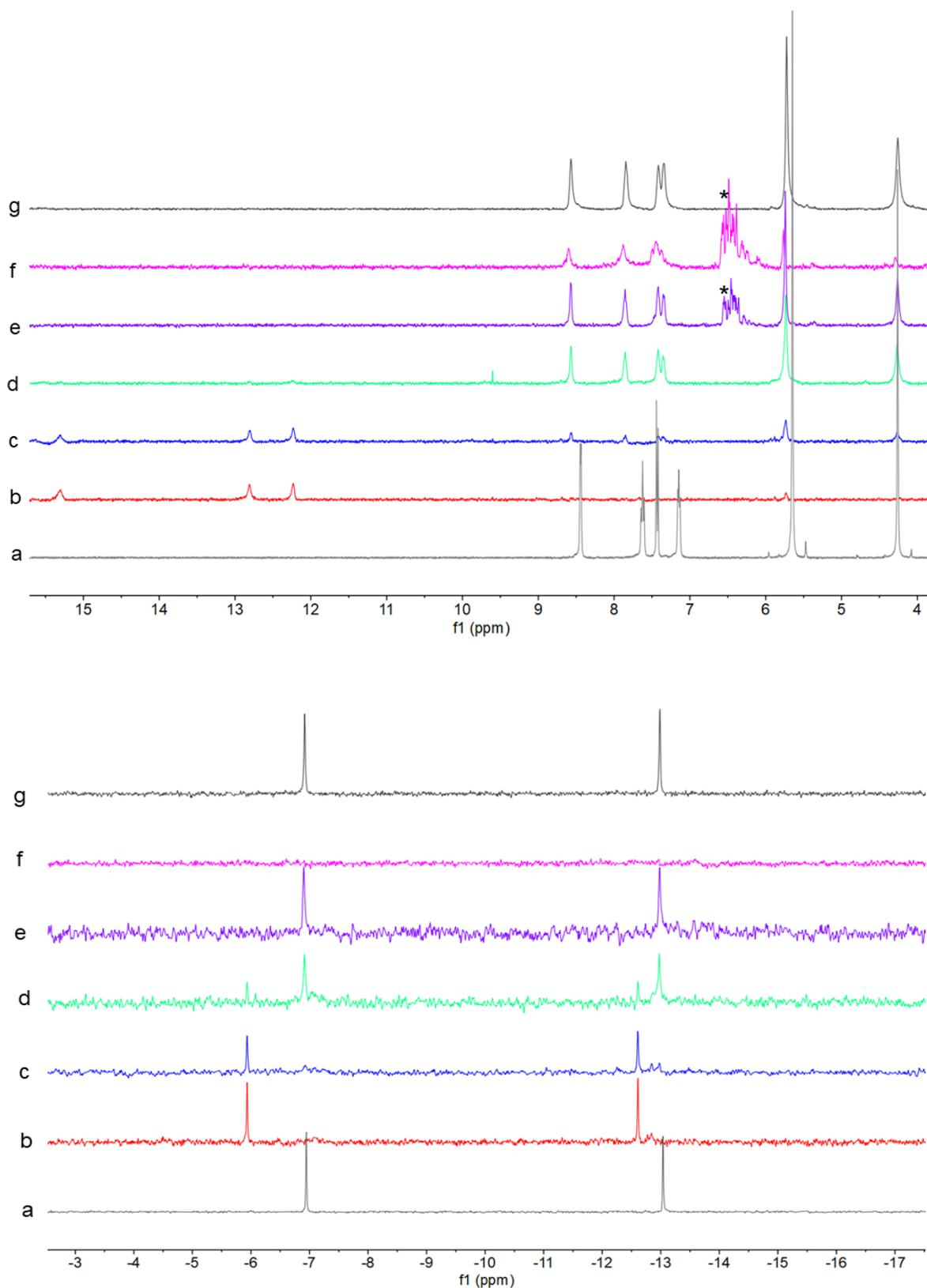
Figure 4-17: A)  $^1H$  NMR spectra and B)  $^{31}P$  NMR of a) ligand  $D_{V3DPA}$  (gray), b) freshly synthesized  $D_{V3DPA}Cu(OAc)$  (red), c) after evolution in the NMR tube (blue), d) after irradiation with a Xenon lamp ( $>385nm$ ,  $75 \mu Wcm^{-1}$ ) (green), e) upon reduction with 1.0 eq.
