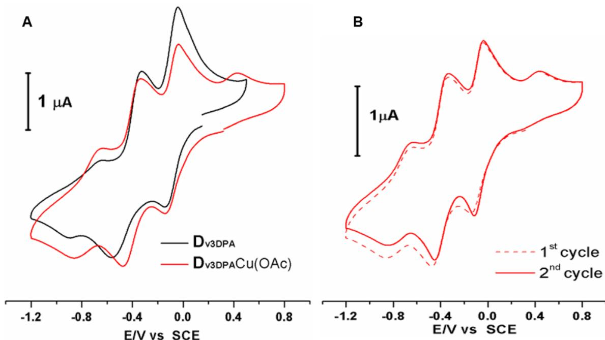
Figure 4-15: A) Cyclic voltammograms of  $D_{V3DPA}$  (black) and  $D_{V3DPA}Cu(OAc)$  (red) at  $1.0 \text{ mmol.L}^{-1}$  in  $CH_3CN$  containing  $0.1 \text{ mol.L}^{-1}$   $TBAPF_6$  and  $v = 100 \text{ mV s}^{-1}$ . B) Cyclic voltammograms of  $D_{V3DPA}Cu(OAc)$  first cycle (dash) and second cycle (solid).
