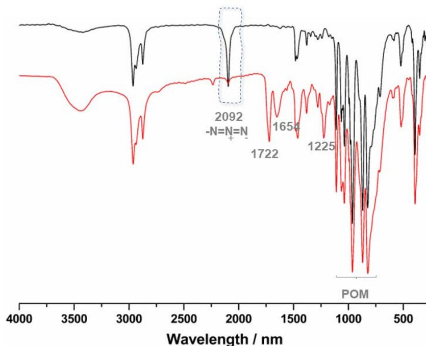
Figure 3-27 Comparison of the IR spectrum of the isolated product  $K_{Si}[MP]-3$  and the starting  $K_{Si}[N_3]-3$ .
