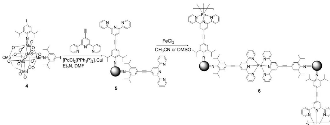
Figure 1-19 Synthesis of transition-metal complexes of POM hybrid-based ligands: dimer and polymer.<sup>57</sup>
