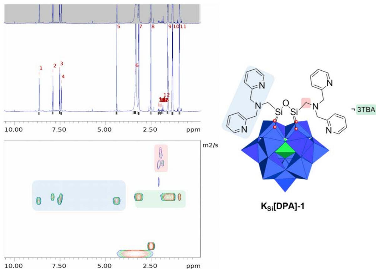
Figure 2-10 The DOSY NMR (in  $\text{DMSO}-d_6$ ) of the synthesized  $\mathbf{K}_{\text{Si}}[\text{DPA}]-1$ .
