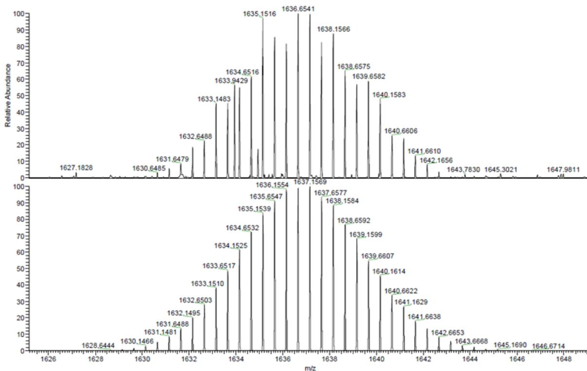
Figure 2-3 ESI-mass spectrum of  $\text{K}_{\text{Si}}[\text{I}]-1$  and its simulation give the formular
