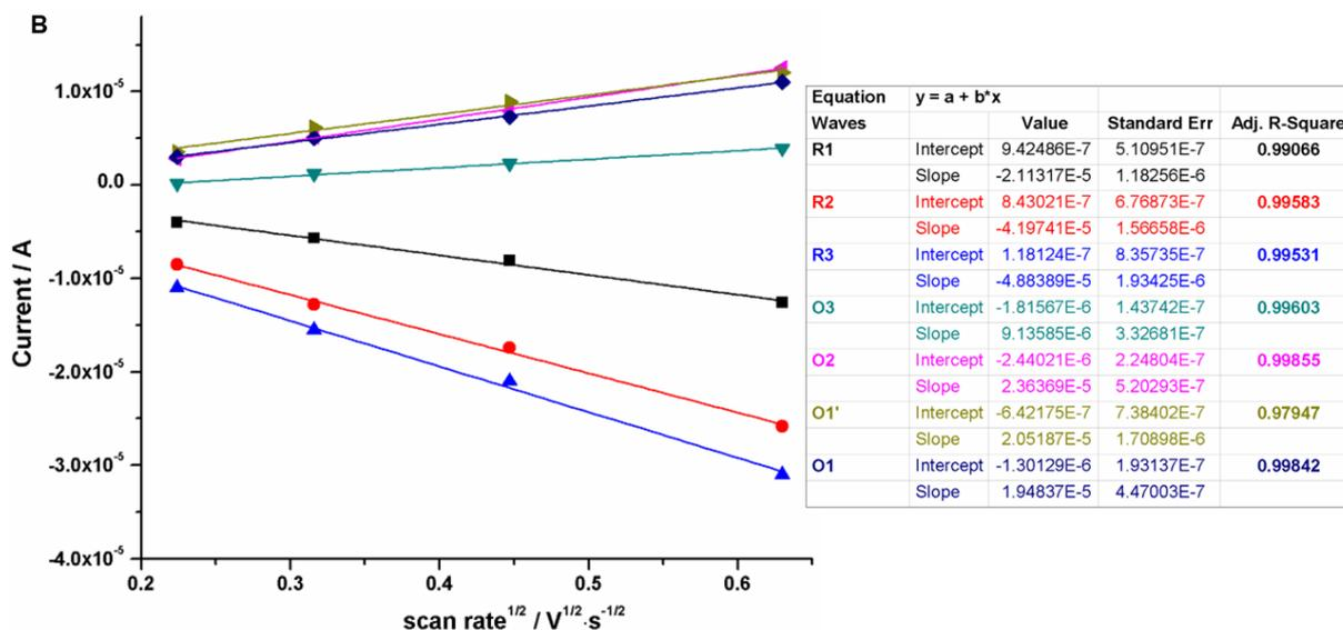
Figure 3-17 A) Cyclic voltammogram of 1.0 mg/mL solution of  $K_{Sn}[DPA]@Cu(OAc)_2$  in MeCN containing 0.1 M of  $TBAPF_6$ , scan rate: 50, 100, 200, 400 mV/s, working electrode: glassy carbon, reference electrode: SCE; B) the slop of current in function of square root of scan rate.
