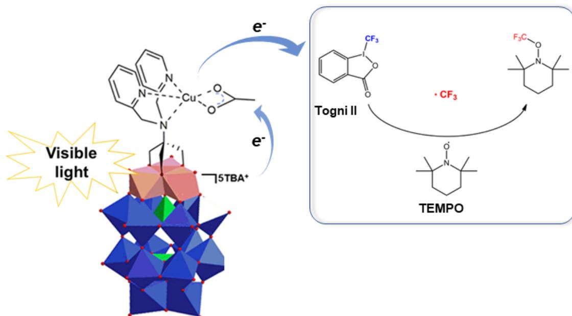
Scheme 4-7 The proposal process of the visible light introduced Cu(II) reduction. TEMPO trapping for the generation of  $CF_3$  radicals
