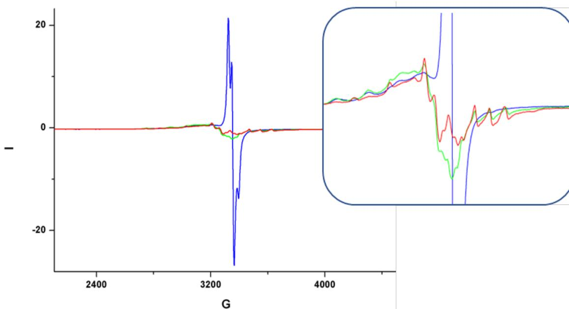
Figure 4-22 EPR spectrum (X-band 9.4GHz 30K) in acetonitrile of TEMPO trapping experiments for the generation of  $CF_3$  radicals with the  $D_{V3DPA}Cu(OAc)$  : TEMPO : Togni II = 1: 1: 2 after 0- (blue), 0.5- (green) and 1-hour (red) irradiation with visible light ( $> 382$  nm).
