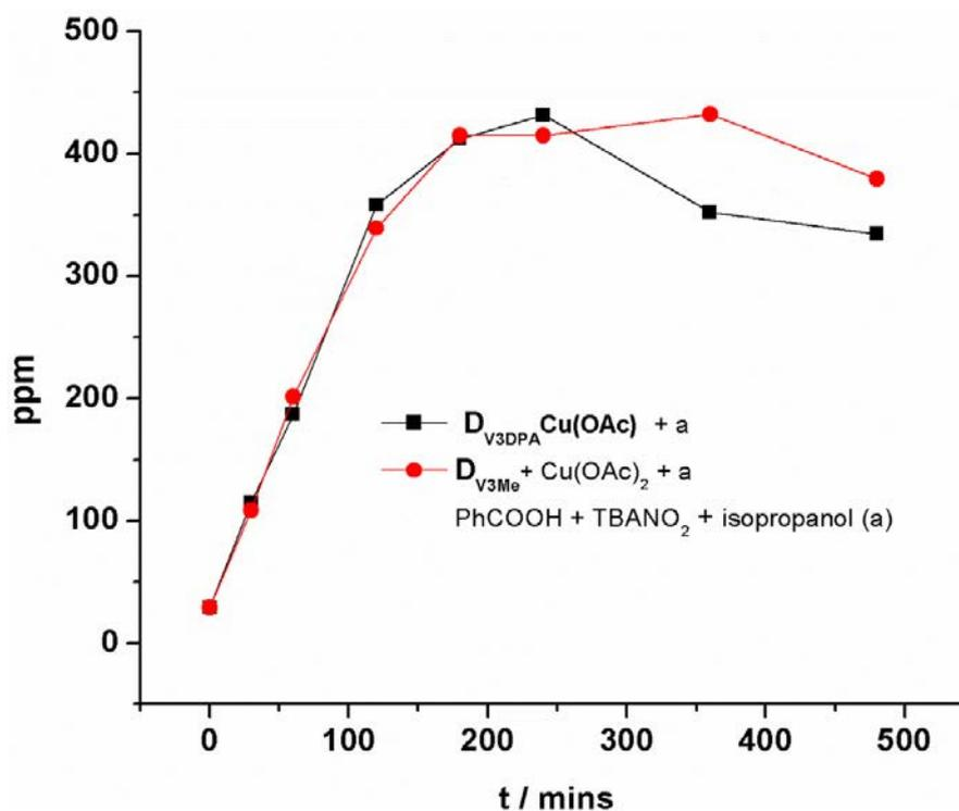
Figure 4-19 Amount of photo-produced NO from  $TBANO_2$  (160eq., 110 mM) in 1.5 mL acetonitrile with the catalyst  $D_{V3DPA} Cu(OAc)$  (0.67 mM) or the mixture of  $[D_{V3Me} + Cu(OAc)_2]$  (0.67 mM) in the presence of benzoic acid (160 eq., 110mM) and isopropanol (160 eq., 110 mM) in function of irradiation time.
