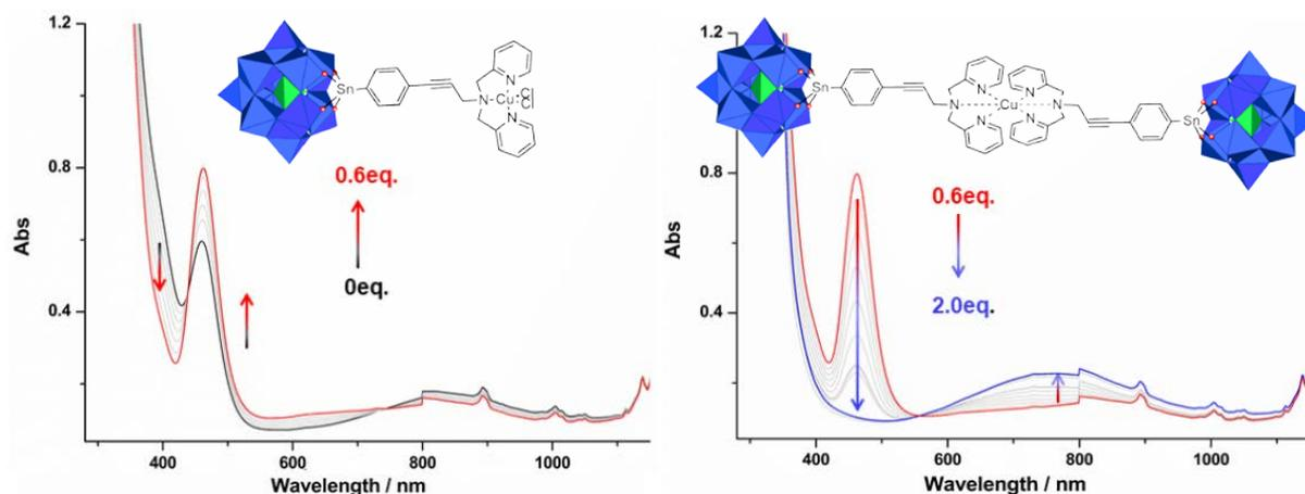
Figure 3-10 The UV-vis titration of 1.0 mM  $\text{CuCl}_2$  with  $\text{K}_{\text{Sn}}[\text{DPA}]$ .
