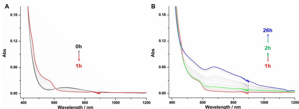
Figure 4-20: Evolution of the UV-VIS signature of a 0.2 mM solution of  $D_{V3DPA}Cu(OAc)$  in acetonitrile upon visible light irradiation. Arrows highlight the successive changes of species associated with photoreduction of the complex by 1, 2 or 3 electrons.
