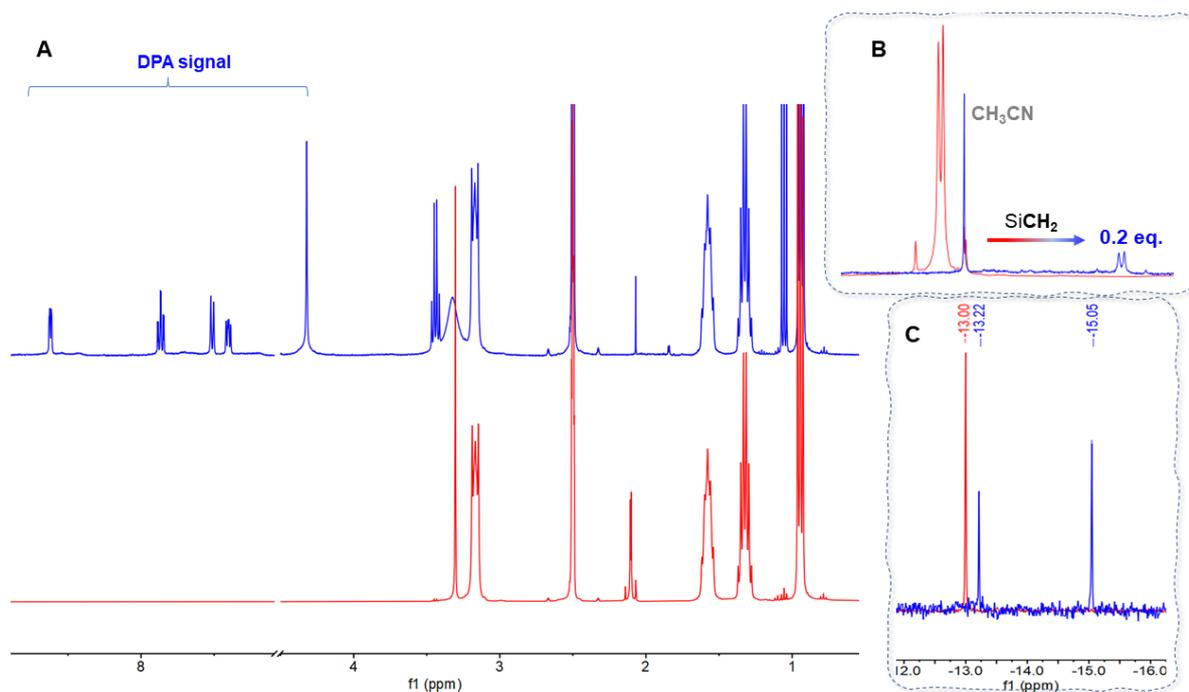
Figure 2-6 The Full range (A) and zoom of the  $\text{SiCH}_2$  (B) of the  $^1\text{H}$  NMR and  $^{31}\text{P}$  NMR(C) spectrum of precursor  $\text{K}_{\text{Si}}[\text{I}]\text{-1}$  (red) and the synthesized  $\text{K}_{\text{Si}}[\text{DPA}]\text{-1}$  (blue).
