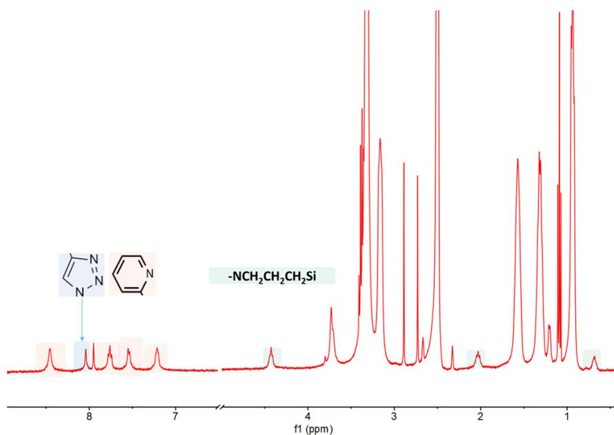
Figure 3-31 the <sup>1</sup>H NMR of the synthesis  $\text{K}_{\text{Si}}[\text{N}_3\text{DPA}]\text{-3}$  with 1.0 eq. of  $\text{CuI}$  and 2.0 eq.  $\text{DIPA}$  heated at 50°C, inset: the <sup>31</sup>P NMR.
