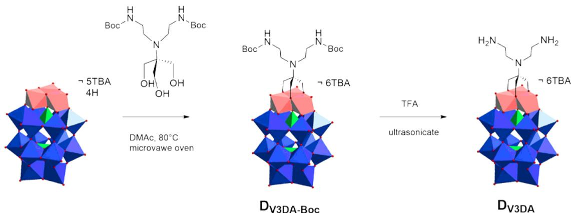
*Scheme 4-4 The synthesis route of  $TBA_6[P_2V_3W_{15}O_{62}(Tris-DA-Boc)]$  (abbreviated **D<sub>V3</sub>DA-Boc**) and  $TBA_6[P_2V_3W_{15}O_{62}(Tris-DA)]$  (abbreviated **D<sub>V3</sub>DA**).*
