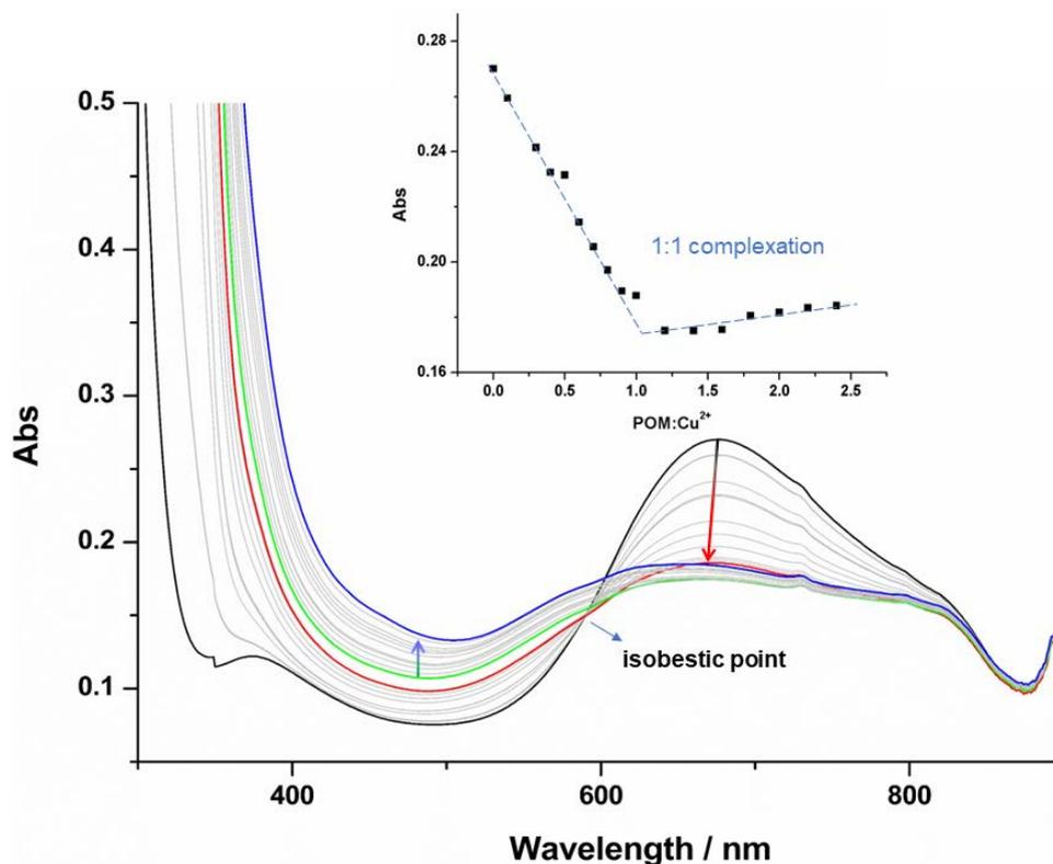
Figure 3-11 The UV-vis titration of the complexation of 1.0 mM  $\text{Cu}(\text{OAc})_2$  with  $\text{KSn}[\text{DPA}]$ .
