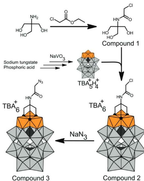
Figure 1-18 The synthesis route to terminal azido functionalized trivanadate substituted Dawson POM, following a with nucleophilic substitution reaction.<sup>55</sup>
