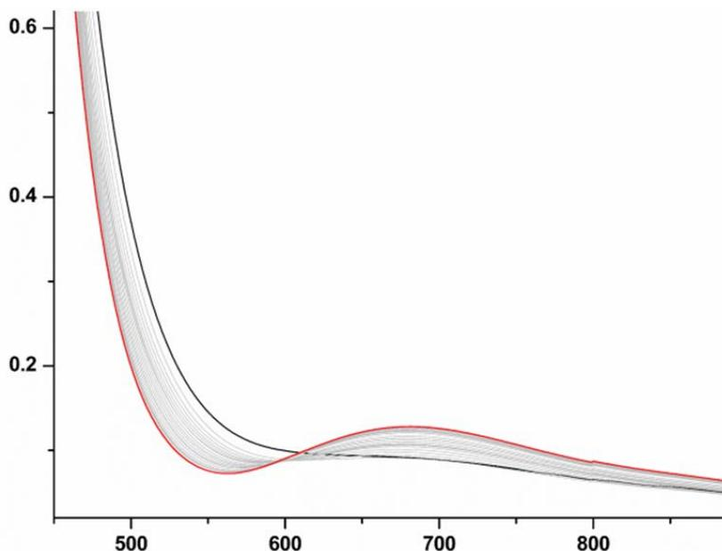
Figure 4-18 UV-vis spectrum of the  $D_{V3DPA}Cu(OAc)$  (1.0 mM) with the titration of peracetate acid from 0 to 2.2 eq.
