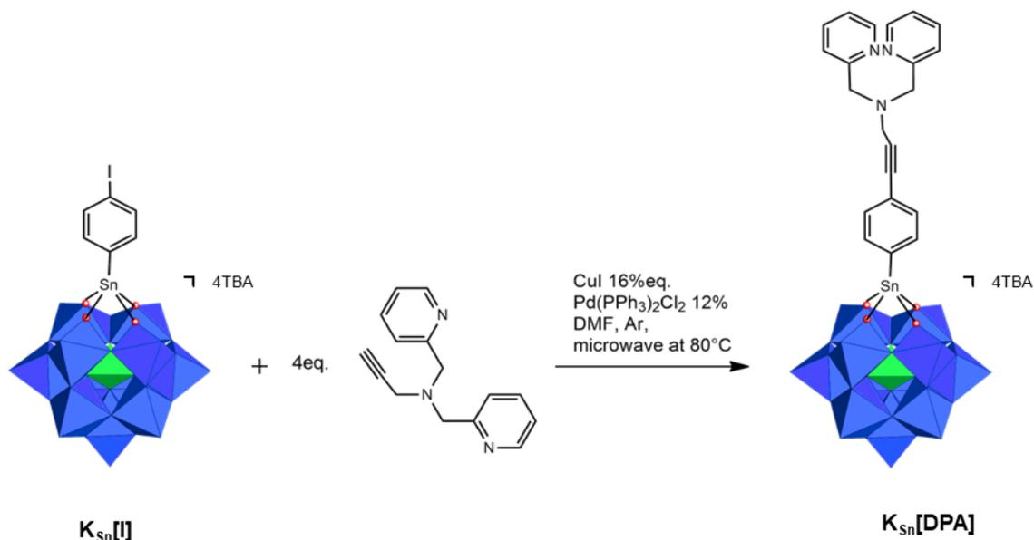
Scheme 3-4 The synthesis of  $TBA_4[PW_{11}O_{39}SnC_6H_4CCCH_2DPA]$  ( $K_{Sn}[DPA]$ )
