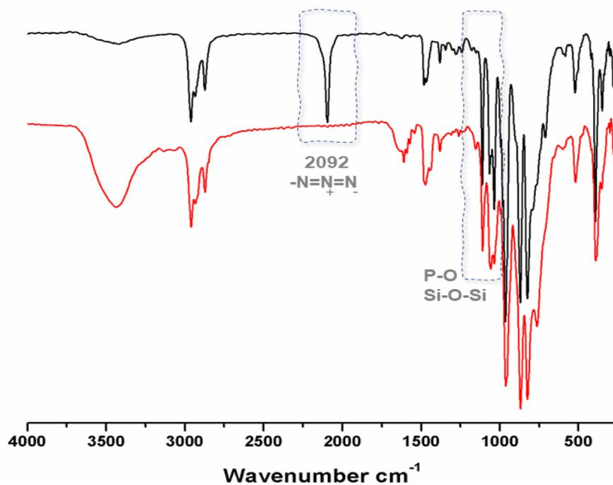
Figure 3-30 The IR spectrum of the synthesis of  $\text{K}_{\text{Si}}[\text{N}_3\text{DPA}]\text{-3}$  with 1.0 eq. of  $\text{CuI}$  and 2.0 eq.  $\text{DIPA}$  heated at 50°C.
