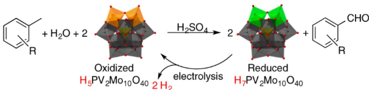
Figure 1-9 The oxidation of methylarenes to benzaldehyde derivatives in aqueous sulfuric acid with  $H_5PV_2Mo_{10}O_{40}$  cycling with electrolysis.<sup>26</sup>
