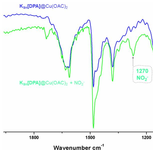
Figure 3-20 IR of the isolated titration product of  $K_{Sn}[DPA]@Cu(OAc)_2$  (green) with  $TBANO_2$ .
