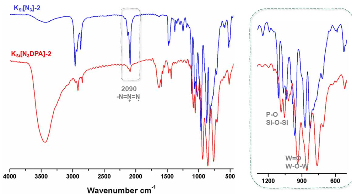
Figure 3-43 The IR spectrum of  $K_{Si}[N_3]-2$  (blue) and  $K_{Si}[N_3DPA]-2$  (red).
