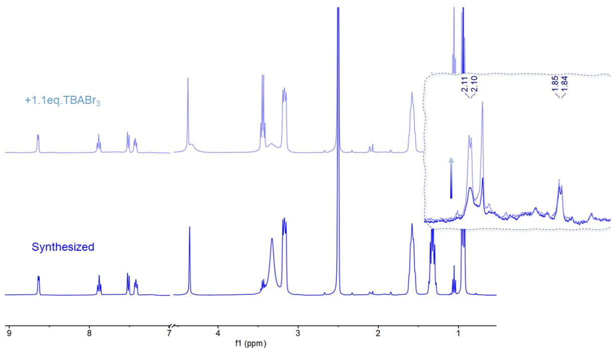
Figure 2-8 the  $^1\text{H}$  NMR (in  $\text{DMSO-d}_6$ ) of the resulting product before (navy) and after (red) the treatment with  $\text{TBABr}_3$ , insert: zoom
