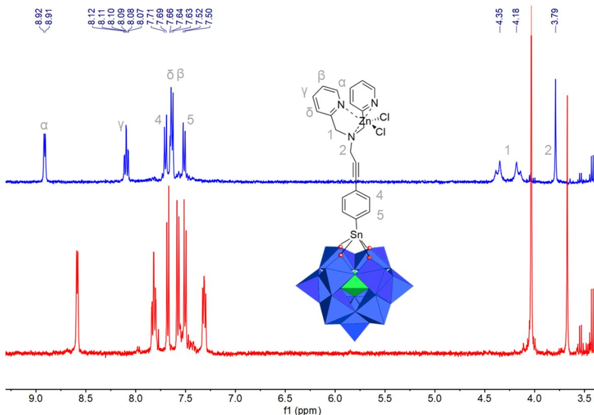
Figure 3-9 The <sup>1</sup>H NMR variation of the  $K_{Sn}[DPA]$  complexation process with  $ZnCl_2$ .
