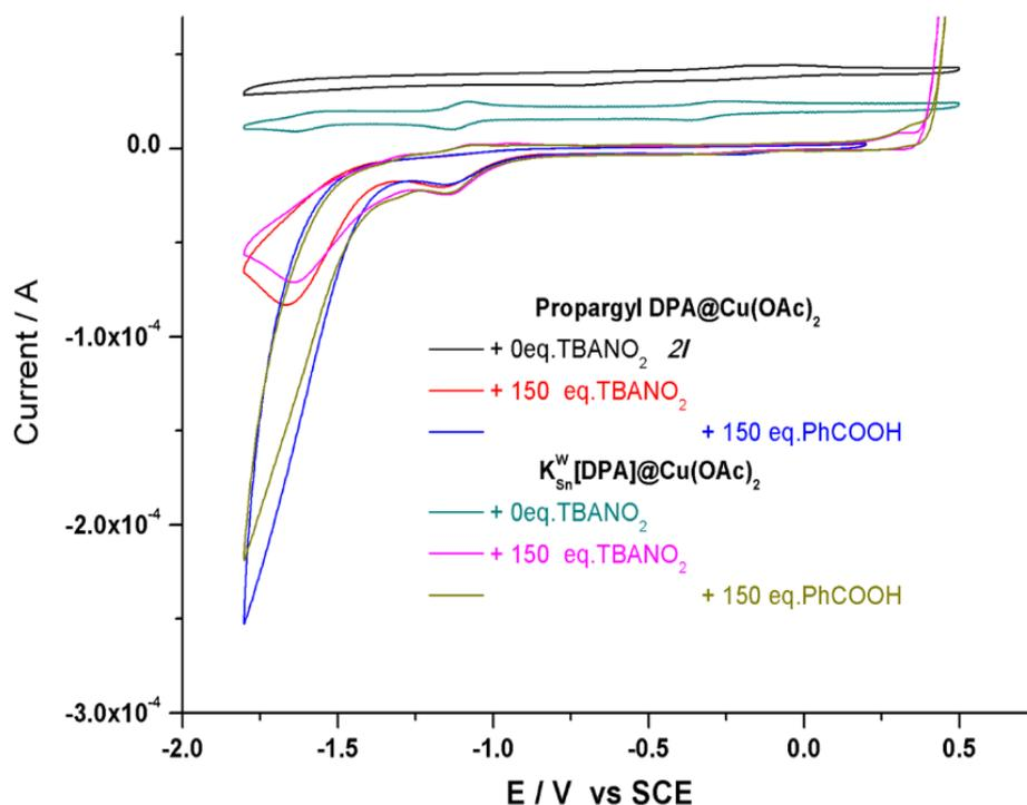
Figure 3-22 Cyclic voltammogram of 0.45 mM solution of  $K_{sn}[DPA]@Cu(OAc)_2$  and propargyl  $DPA@Cu(OAc)_2$  respectively, with or without the presence of 150 eq.  $TBANO_2$  and 150 eq.  $PhCOOH$ , in degassed DMF containing 0.1 M of  $TBAPF_6$ , scan rate: 100 mV/s, working electrode: glassy carbon, reference electrode: SCE.
