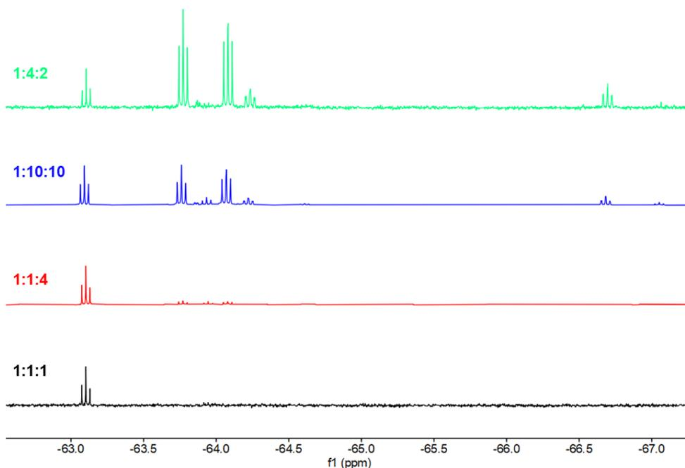
Figure 4-25 Evolution of the  $^{19}F$  NMR as a function of the ratio styrene to Togni II 1:1, 1:4 (red), 10:10 (green), 4:2 (blue).
