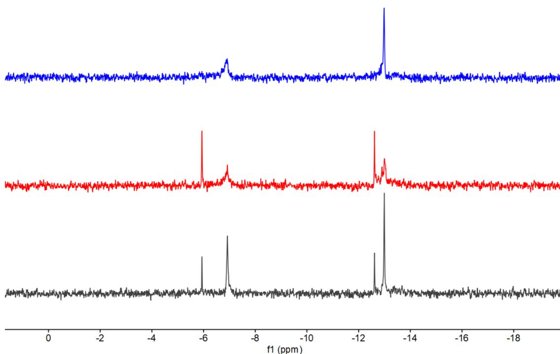
Figure 4-15 The  $^{31}P$  NMR of the partly photo-reduced  $D_{V3DPA}\{Cu^{II}(OAc)$  (black), after addition of  $TBANO_2$  (red) and following irradiation (blue).
