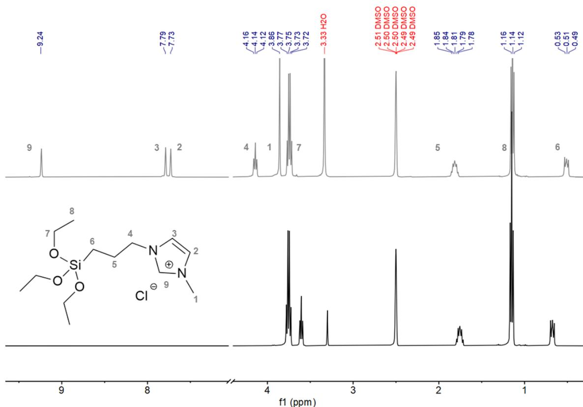
Figure 2-11 The evolution in  $^1\text{H}$  NMR of synthesis of 1-(tri-ethoxy-silyl-propyl)-3-methyl-imidazolium chloride (gray) from the solvent-free reaction of (3-chloropropyl)triethoxysilane (black) and 1-methyl-1H-imidazole (**NMI**).
