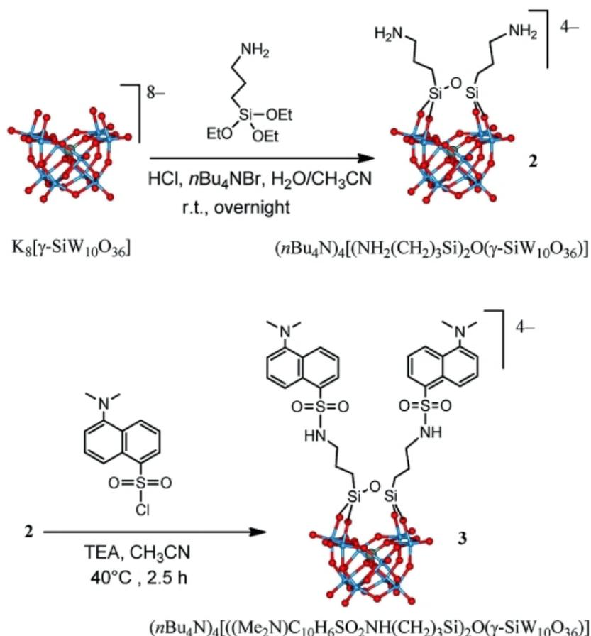
Figure 1-12 The synthesis route of  $\text{NH}_2$ -terminated hybrid  $[\gamma\text{-SiW}_{10}\text{O}_{36}\{\text{O}(\text{Si}(\text{CH}_2)_3\text{NH}_2)_2\}]^{4-}$  and its post-sulfonamidation.<sup>40</sup>
