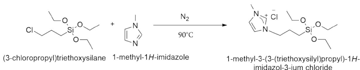
*Scheme 2-9 The synthesis of 1-(tri-ethoxy-silyl-propyl)-3-methyl-imidazolium chloride*
