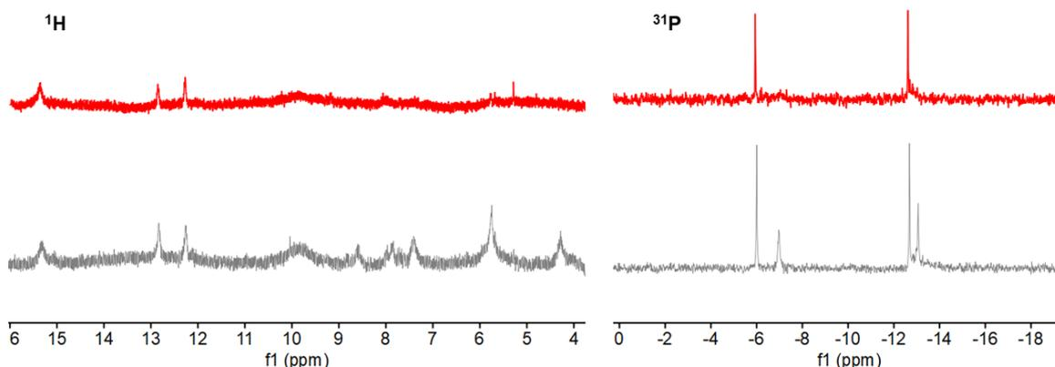
Figure 4-19  $^1H$  NMR and  $^{31}P$  NMR of  $D_{V3DPA}Cu(OAc)$  before (gray) and after (red) being oxidized by peracetate acid 2.0 eq.
