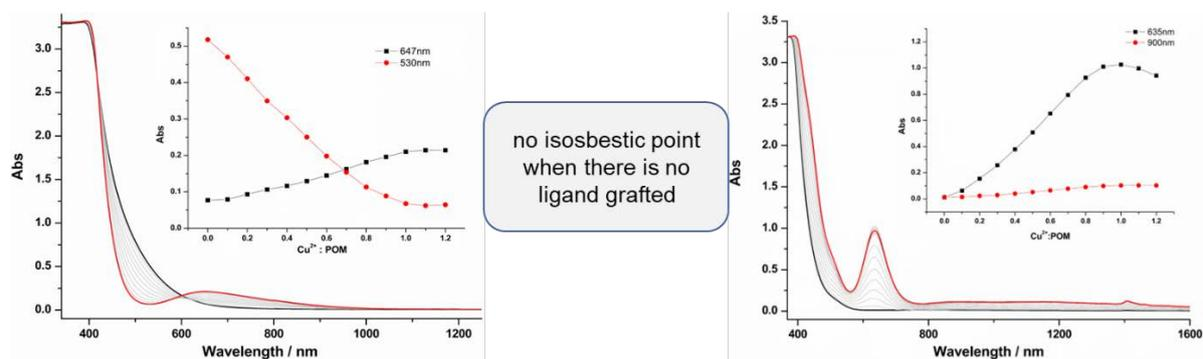
Figure 4-35 UV-vis titration of  $D_{V3DPA}$  and  $D_{V3}$  with  $Cu(ClO_4)_2$
