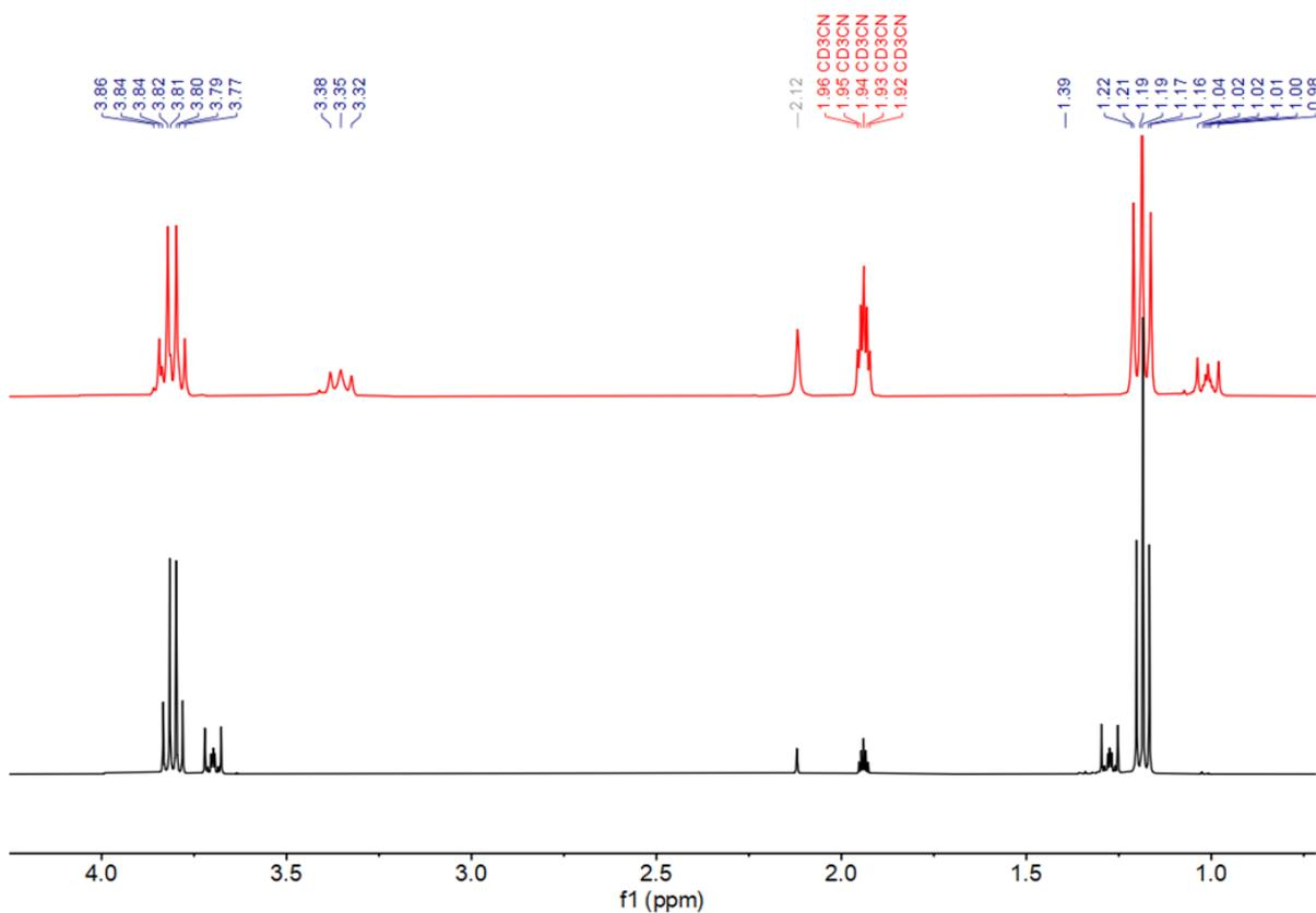
Figure 3-39 The  $^1\text{H}$  NMR of 2-azidoethyl triethoxysilan (red) and the precursor 2-chloroethyl triethoxysilan (black) in  $\text{CD}_3\text{CN}$ .
