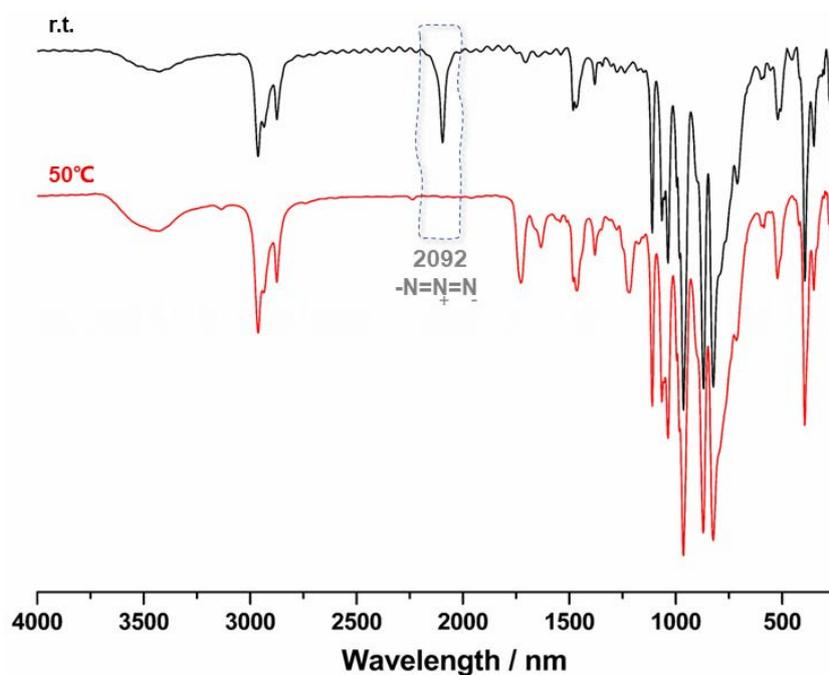
Figure 3-29 IR monitor of the “click” between  $K_{Si}[N_3]-3$  and methyl propiolate in the presence of 2.0 eq. DIPA at room temperature (black) and 50°C (red).
