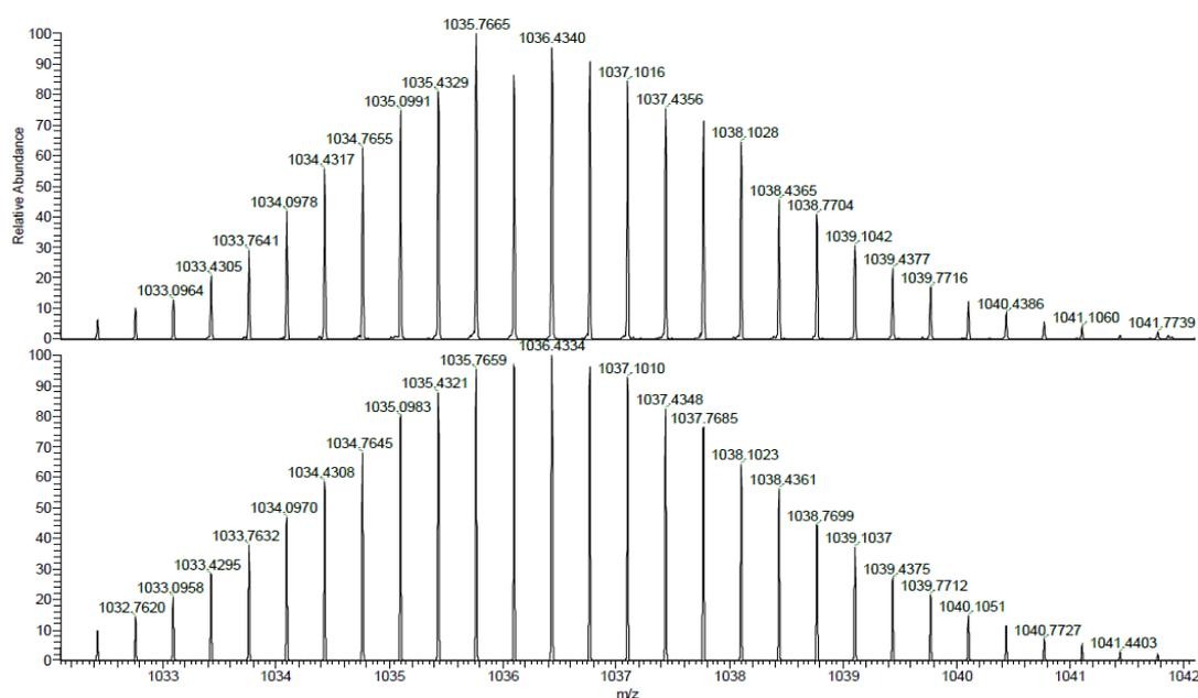
Figure 3-8 The ESI-MS of  $\text{K}_{\text{Sn}}[\text{DPA}]$  which gives the formula  $\{\text{HK}_{\text{Sn}}[\text{DPA}]\}^{3-}$ .
