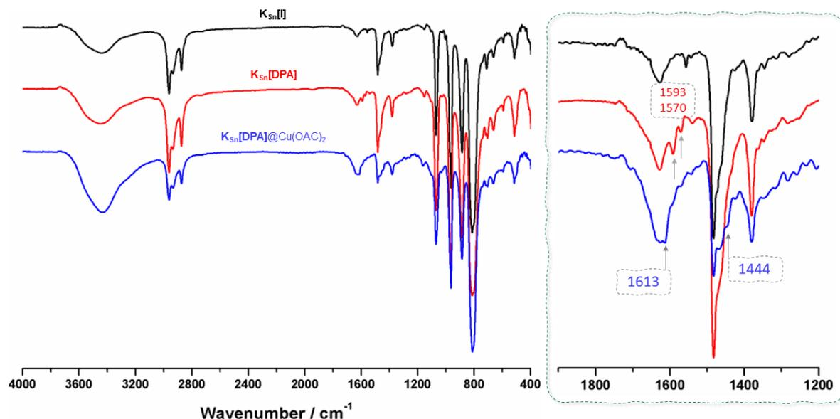
Figure 3-15 The normalized infrared spectrum of precursor platform  $K_{Sn}[W]$  (black), the ligand  $K_{Sn}[DPA]$  (red) and the complex  $K_{Sn}[DPA]@Cu(OAc)_2$  (blue).
