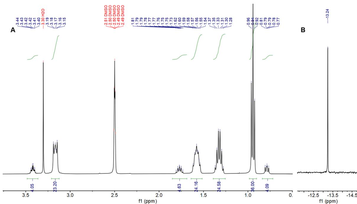
Figure 3-24 the  $^1H$  NMR of  $K_{Si}[N_3]-3$  in DMSO and the  $^{31}P$  NMR.
