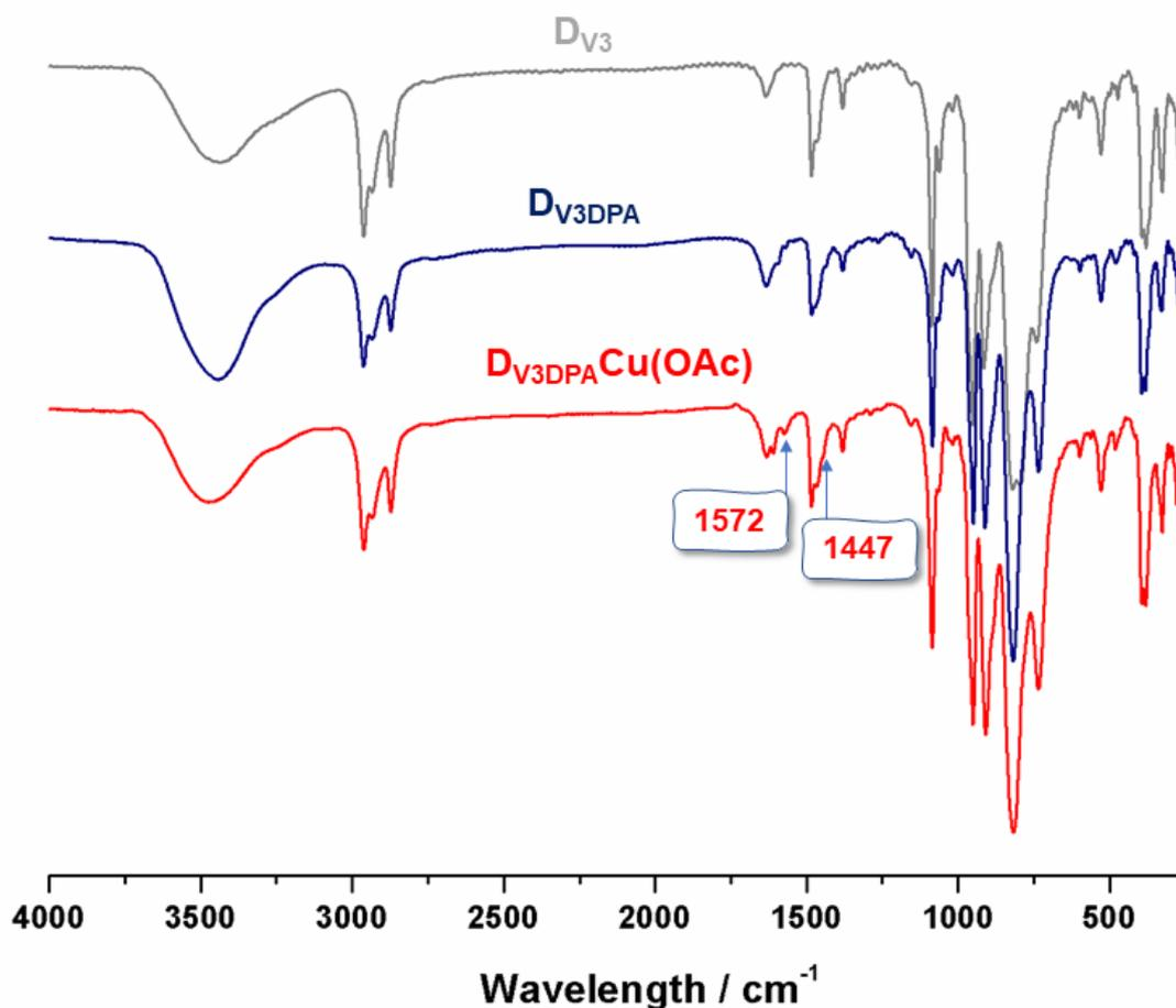
Figure 4-11 the IR of  $D_{V3}$  (gray),  $D_{V3DPA}$  (navy blue) and  $D_{V3DPA}Cu(OAc)$  (red). The arrows point out the absorption of acetate  $1572\text{ cm}^{-1}$  and  $1447\text{ cm}^{-1}$
