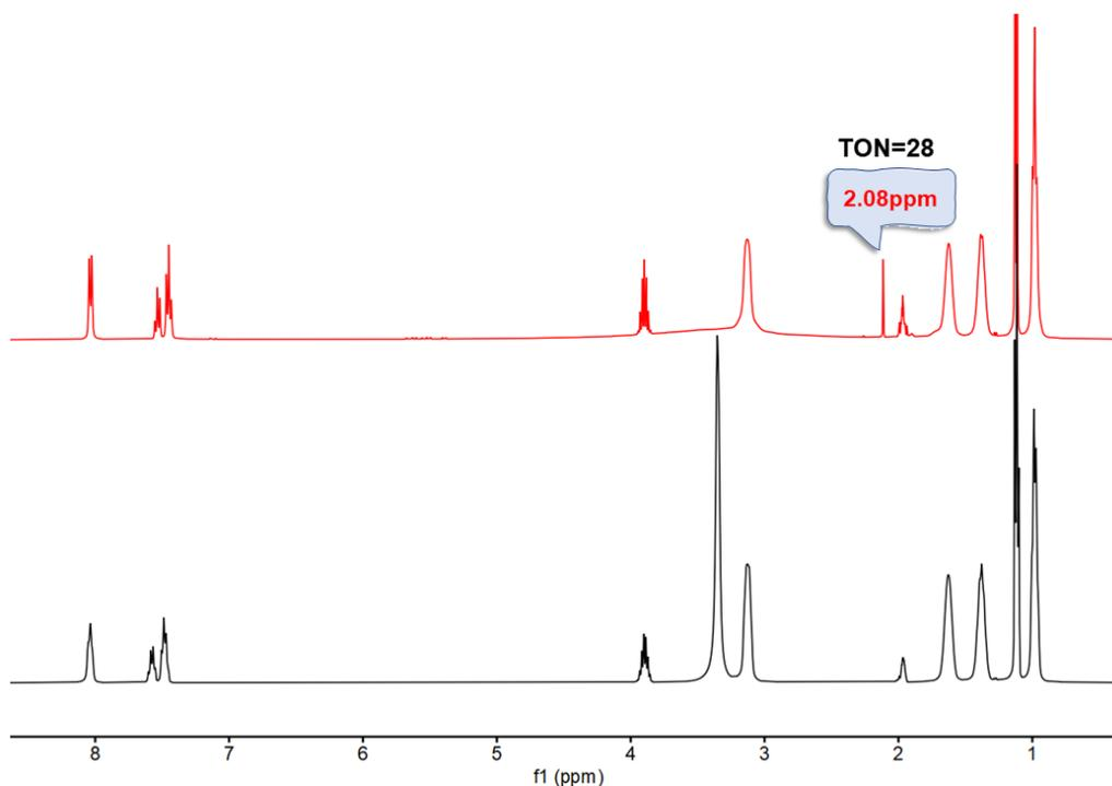
Figure 4-16 The  $^1H$  NMR of  $D_{V3DPA}Cu(OAc)$  (1.0 mM) in the presence of 40 mM of  $TBANO_2$ ,  $PhCOOH$  and isopropanol before and after irradiation with visible light ( $>382$  nm).
