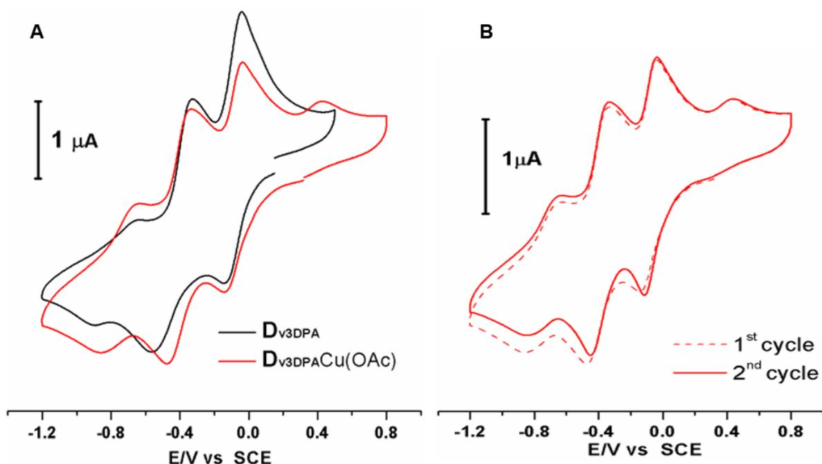
Figure 4-15: A) Cyclic voltammograms of  $D_{V3DPA}$  (black) and  $D_{V3DPA}Cu(OAc)$  (red) at  $1.0 \text{ mmol.L}^{-1}$  in  $CH_3CN$  containing  $0.1 \text{ mol.L}^{-1}$   $TBAPF_6$  and  $v = 100 \text{ mV s}^{-1}$ . B) Cyclic voltammograms of  $D_{V3DPA}Cu(OAc)$  first cycle (dash) and second cycle (solid).
