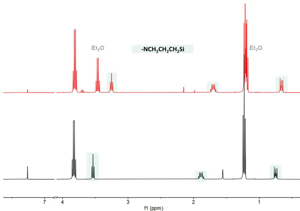
Figure 3-23 the  $^1\text{H}$  NMR of the 3-azidopropyl triethoxysilane (red) and the precursor 3-chloropropyl triethoxysilane ( $\text{CDCl}_3$ )
