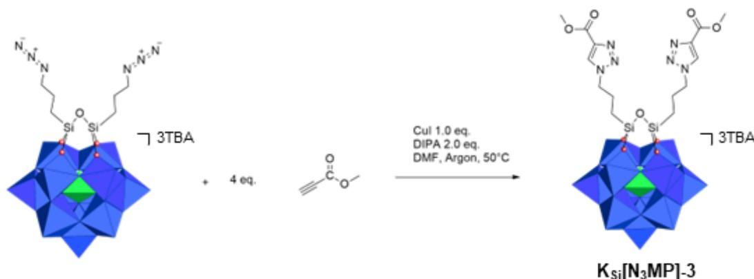
Scheme 3-8 The synthesis of  $\text{K}_{\text{Si}}[\text{N}_3\text{MP}]-3$  in with CuI as catalyst.
