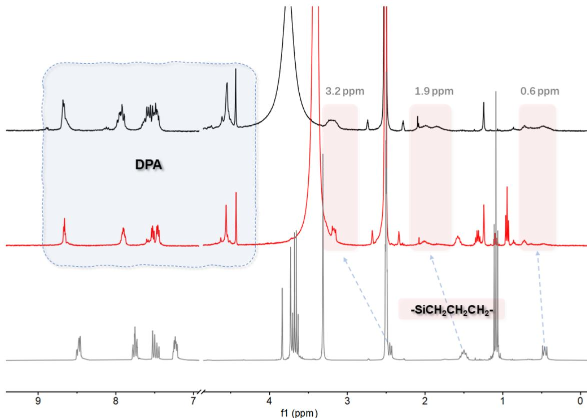
Figure 2-15 The  $^1\text{H}$  NMR of the direct-functionalization of  $\text{K}_{\text{Si}}[\text{DPA}]\text{-3}$  in solvent  $\text{CH}_3\text{CN}:\text{H}_2\text{O}=10:1$  (red) and  $\text{CH}_3\text{CN}:\text{H}_2\text{O}=1:15$  (black) compared to the organic precursor *N,N*-bis(pyridin-2-ylmethyl)-3-(triethoxysilyl)propan-1-amine (gray).
