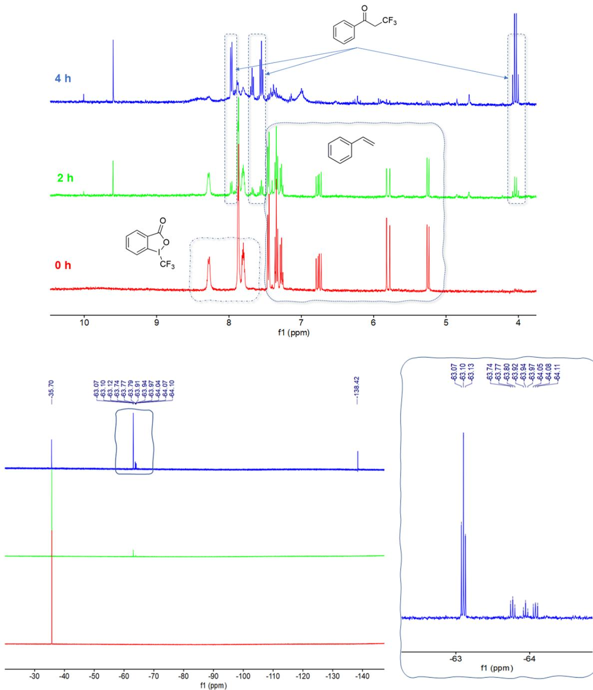
Figure 4-24  $^1H$  NMR and  $^{19}F$  NMR of the reaction of trifluoromethylation of styrene in the ratio of  $D_{V3DPA}Cu(OAc)$ : styrene:  $CF_3^+$  = 1: 1 :4 in  $CD_3CN$  after 0-, 2- and 4-hour irradiation with visible light ( $> 382$  nm).
