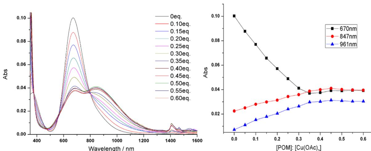
Figure 3-36 The UV-vis titration of 0.50 mM  $\text{Cu}(\text{OAc})_2$  with  $\text{KSi}[\text{N}_3\text{DPA}]-3$  in acetonitrile and the slope at 670, 847 and 961nm.
