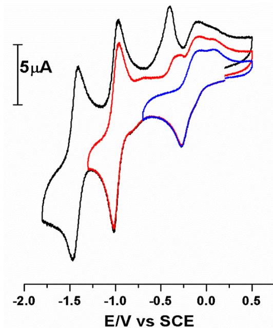
Figure 3-16 Cyclic voltammogram of 1.0 mg/mL solution of  $K_{Sn}[DPA] @Cu(OAc)_2$  with different scan windows: 1) 0.5 to -0.7 V (blue); 2) 0.5 to -1.3 V (red); 3) 0.5 to -1.8 V (black) in MeCN containing 0.1 M of  $TBAPF_6$ , scan rate: 100 mV/s, working electrode: glassy carbon, reference electrode: SCE.
