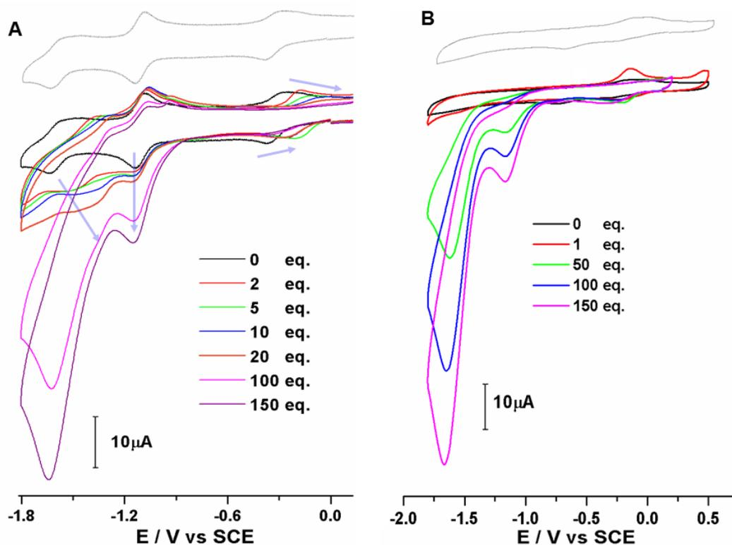
Figure 3-21 Cyclic voltammogram of A) 0.45 mM solution of  $\text{K}_{\text{Sn}}[\text{DPA}]\text{@Cu}(\text{OAc})_2$  in the presence of (0, 2, 5, 10, 20, 100, 150 eq.)  $\text{TBANO}_2$ ; B) 0.45 mM solution of propargyl  $\text{DPA@Cu}(\text{OAc})_2$  in the presence of (0, 1, 50, 100, 150 eq.)  $\text{TBANO}_2$  in degassed DMF containing 0.1 M of  $\text{TBAPF}_6$ , scan rate: 100 mV/s, working electrode: glassy carbon, reference electrode: SCE.
