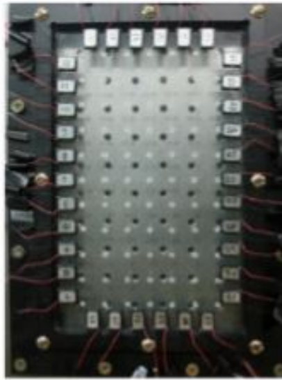
Figure 1.7.: Illustration of the prototype for vibration rendering on a thin plate. Source: image from [19]
