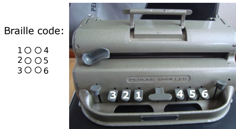
Figure 3.5.: Perkins machine. Source: image from Catawiki [24]
