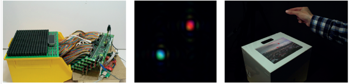
Figure 1.1.: The UltraHaptics system: Left: the setup. Centre: an example of two focal points in the air. Right: user receiving two independent stimulation. Source: images from [13].
