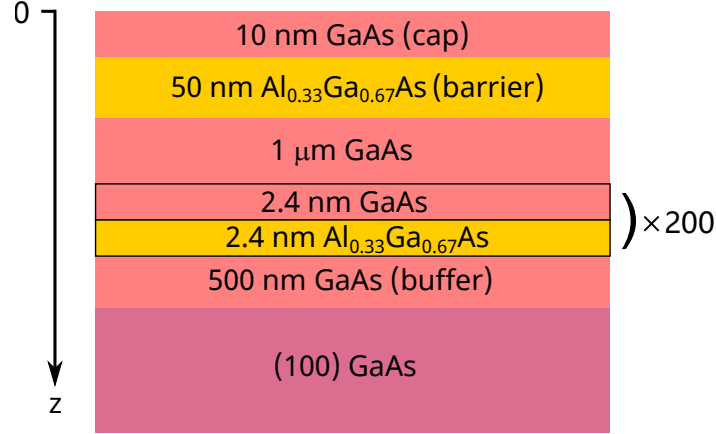
Figure 7.1: Substrate structure for quantum dot device. Above the (100) GaAs wafer (purple) are epitaxial \text{Al}_{0.33}\text{Ga}_{0.67}\text{As} (yellow) and GaAs (red) layers grown by MBE.
