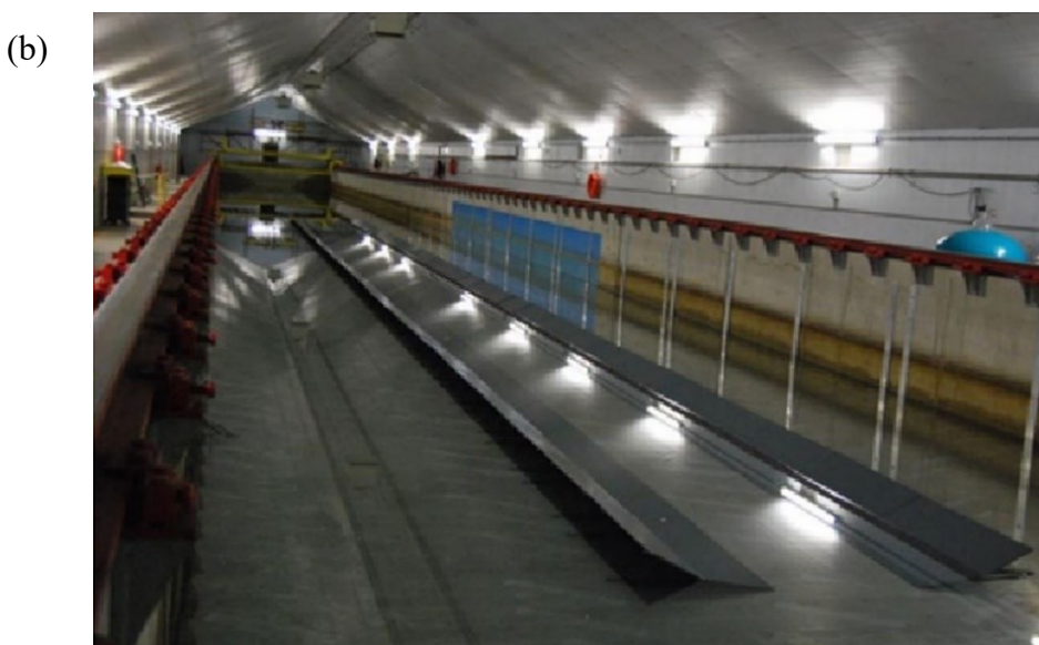
Fig 3. 20 Towing tank for shallow and restricted experiments in Liege university
