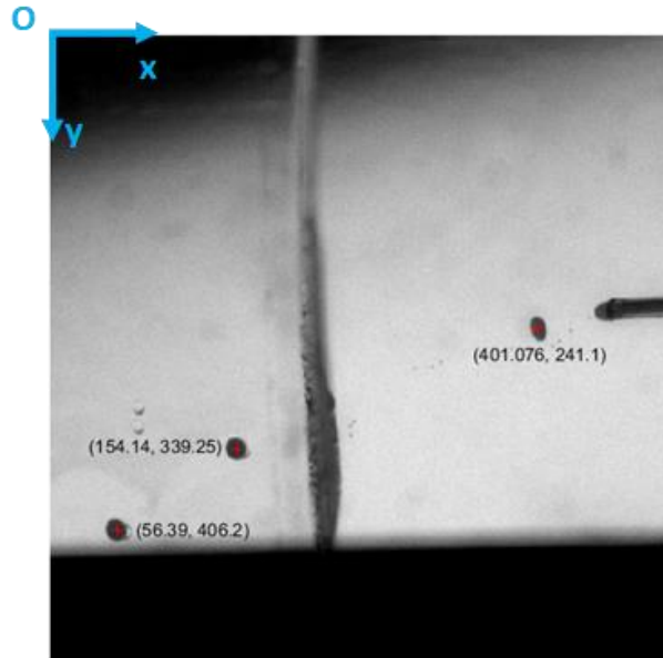
Figure 61: The centers of mass of droplets detected by Hough transforms with their corresponding coordinates in the reference of the image shown on top of the image.
