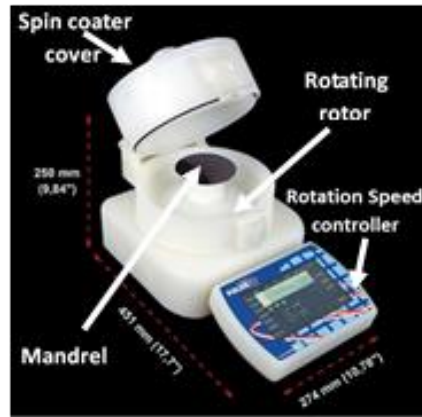
Figure 115: The image of the spin coater from the website of supplying company.
