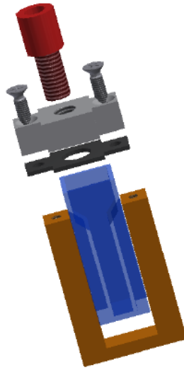
Figure 120: The reservoir and encapsulation cell. In yellow: an aluminum support which will touch the screw connecting the two rectangular supports (top and bottom), in blue: the cells which contains the liquids, in black: a joint to prevent leakage, in grey: a plug to be screwed with the support at its two sides with a hole in the middle permitting the passage of the connecting capillary tube.
