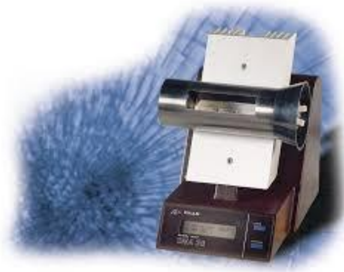
Figure 127: The image of the denismeter used to measure the densities of the samples in this work.
