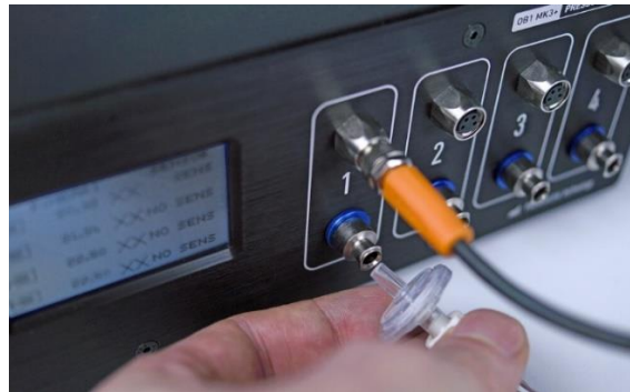
Figure 124: The outlet channel of the pressure regulator where air exits at a controlled pressure.
