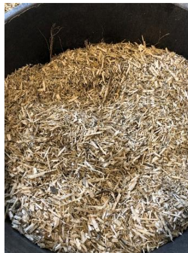
Figure III-12. Bark recovered after the purification process
