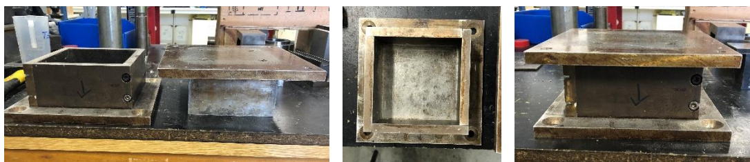
Figure III-13. Mold used for the production of the acoustic panels
