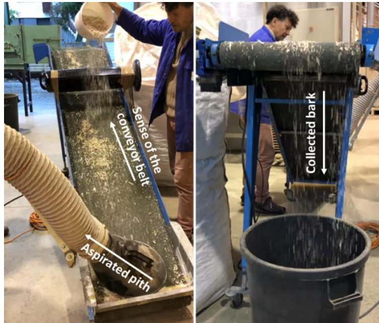
Figure III-10. Conveyor belt and aspiration system put together for the purification process
