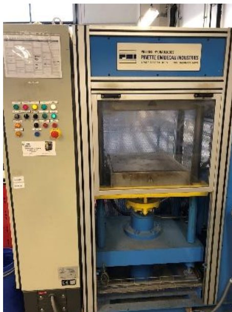
Figure III-14. Heat press used for the production of the water vapor acoustic panel
