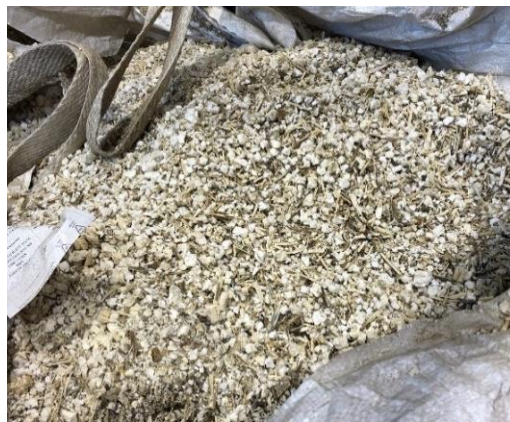
Figure III-6. Crushed stems after passage by the hammer mill
