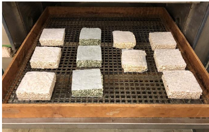
Figure III-19. Insulating panels in the oven for drying
