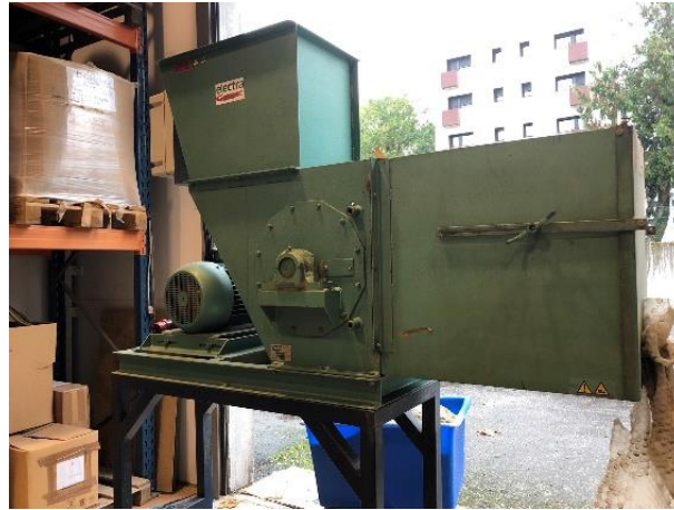
Figure III-5. Hamer mill used for the crushing of the sunflower stems
