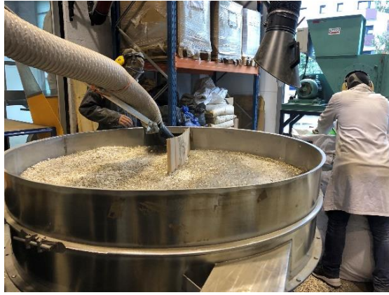
Figure III-7. Sieve and aspiration system used in the separation process
