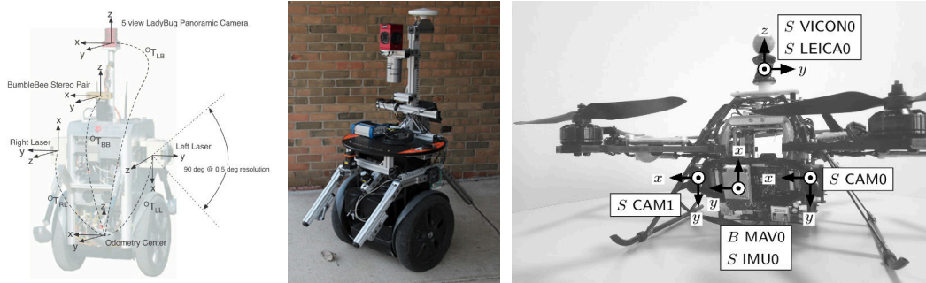
Figure 7.6: Mobile robots used for SLAM datasets. From left to right, the Segway platform used in the New College dataset [198], the Segway platform used in the NCLT dataset [35], the MAV used in the EuRoC MAV dataset [30].
