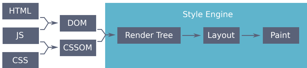
Figure 3.3: Rendering process of a Web page.
