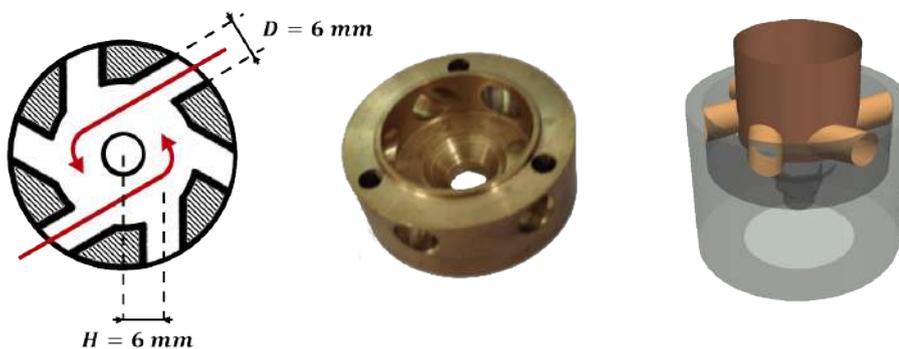
Figure 3.3: Top view sketch of the swirler used in this work (left), real swirler geometry (middle) and 3D rendering of the swirler as used in numerical simulations (right).
