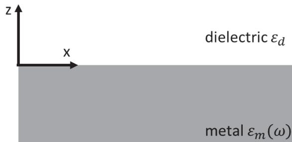
Figure 1.5: **Schematic representation of a surface plasmon propagating along the dielectric interface/metal.**  $\epsilon_d$  and  $\epsilon_m(\omega)$  are the relative dielectric function of the dielectric and metal, respectively.
