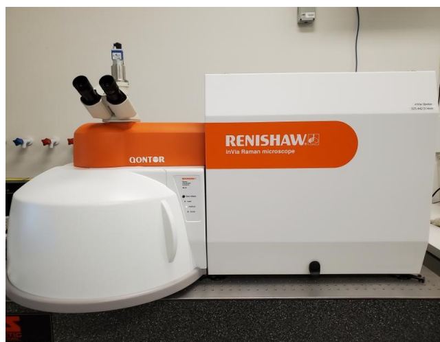
Figure 2.9: Renishaw In-Via spectrometer for Raman Spectroscopy measurements.
