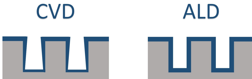
Figure 1.11: Difference between CVD and ALD in uniformity and conformality distribution over 3D substrate area.
