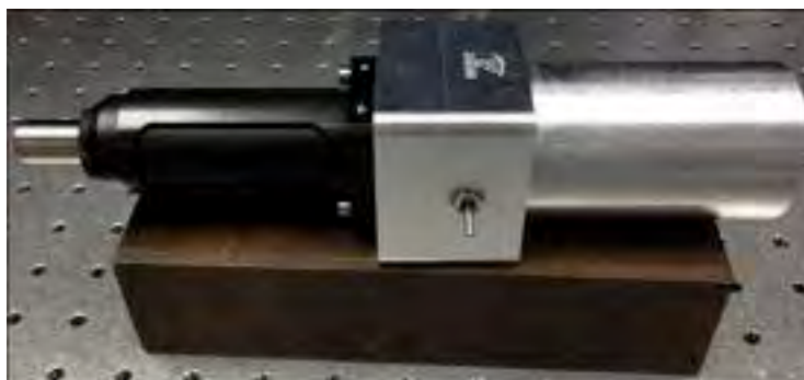
Fig. 3. Handheld part of the 1-shot OFI system for single point acquisition.
