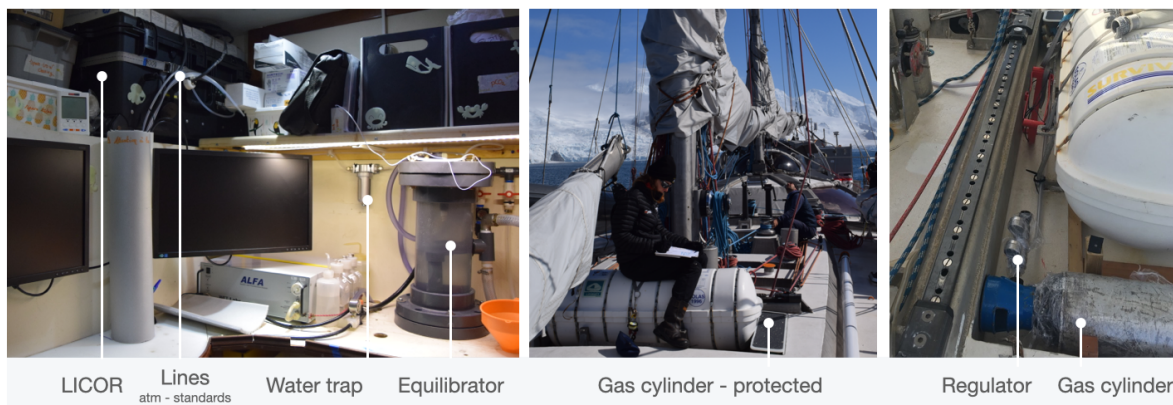
Figure 3.6: f\text{CO}_2 sampling devices on-board SV Tara. The picture on the left shows the interior of the underway laboratory, where the equilibrator and the LICOR (inside the black box) are installed. The atmospheric and standards lines connect directly to the black box. The middle picture shows the front deck of the ship, the standards (gas cylinders) are laying on each side of the life raft, protected by an anti-slip plastic support. Right: the support is removed, the gas cylinder, the regulator and the lines are apparent.
