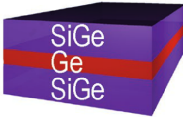
Figure 1: Schematic of the Ge/SiGe heterostructure. Figure taken from [26].
