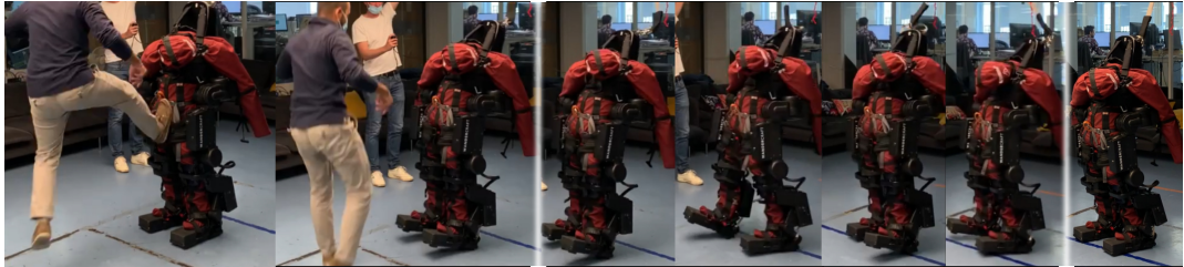
Figure 6.7: Strong impact kick, 1 recovery step per frame in the highlighted section.
