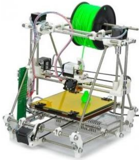
Figure 3: Picture of a basic RepRap printer [23]
