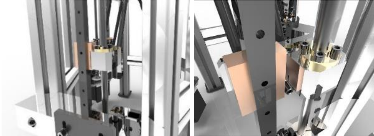
Figure 13: Linear guide rail marks as n. 3 in the 3D stage assembly
