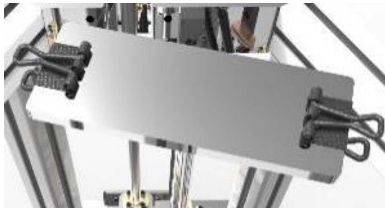
Figure 11: Deposition platform marks as n. 1 in the 3D stage assembly
